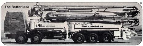
The Putzmeister M 52 with 200 cubic yards per hour capacity, 360 HP engine, on the road to Chernobyl with its lead lined cab. The compact five section Multi-Z-Boom was fully automatic, centrally lubricated, all radio and video controlled, including S-type harsh mix hopper to match most difficult concrete mixes.
