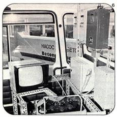
Video monitoring in the driver's cab, parallel to same installation positioned 2,000 ft. away in a protective control centre for all pumps.
