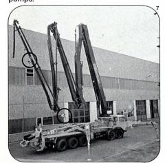
Camera at the fifth section surveys concrete distribution. Multi-Z for low unfolding height. End hose is immediately in service without long fold-out process. Second lead-lined video camera automatically extends when outriggers swing out to survey hopper functions.
