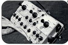
Radio remote control for all functions including outriggers In/Out, engine Start/Stop, all volume controls, etc. In addition to this, cable remote control was installed as an alternative to increase redundancy – also because nobody knew if the radio control would function under radioactive radiation.
