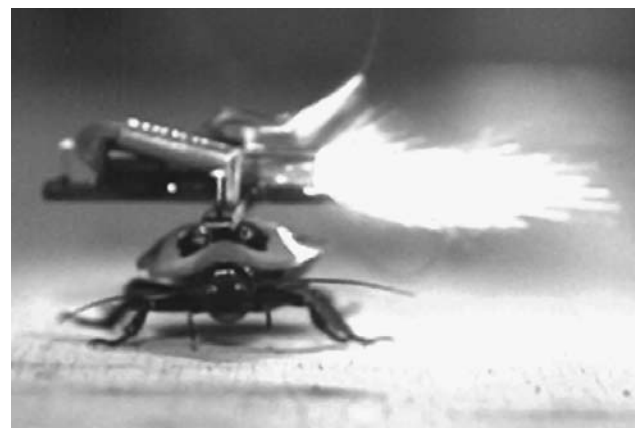
Fig. 2.2 Blaberus discoidalis with an exploding cannon backpack attempting to knock it off balance. Photo courtesy of Devin Jindrich.
