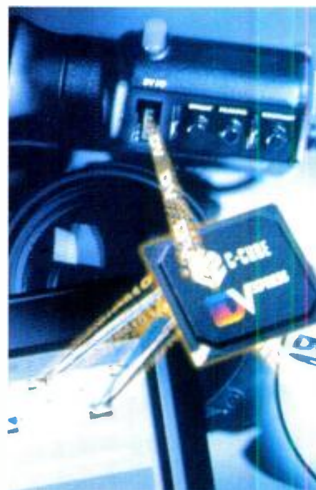
C-Cube's DVxpress-MX chip will act as a bridge between the DV and MPEG-2 formats.
