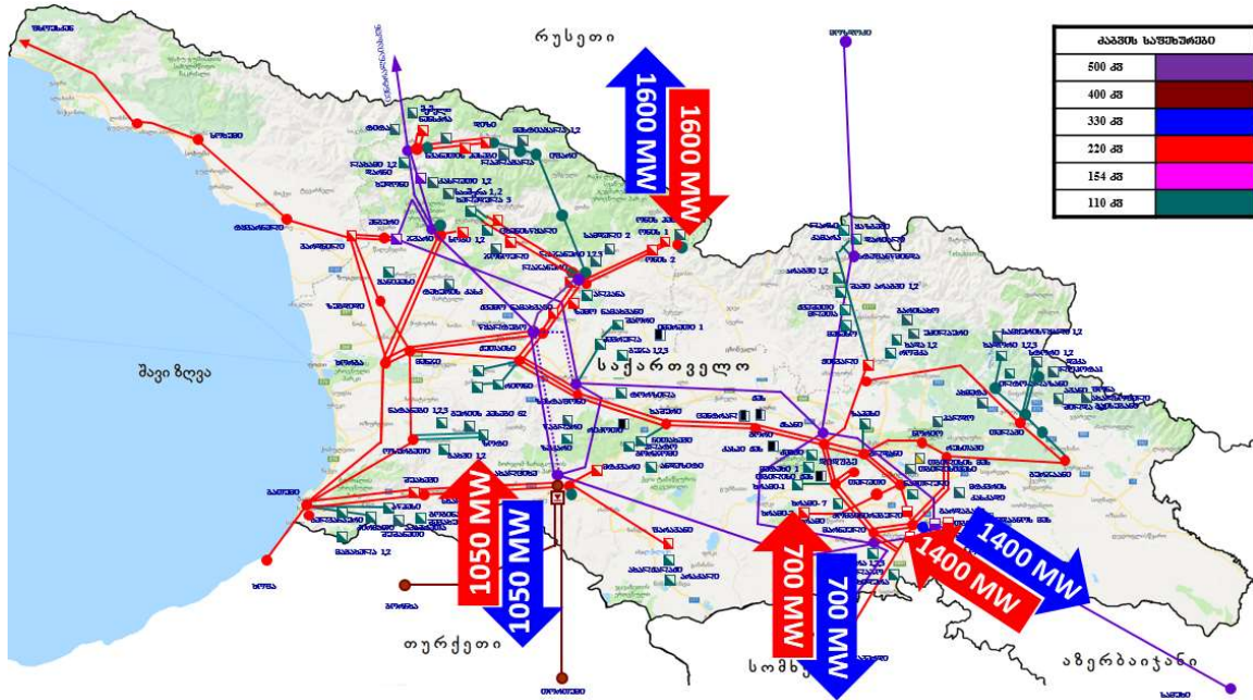
Fig. 1.12 Cross-border transfer capacities between power systems of Georgia and its neighboring countries as for 2032
