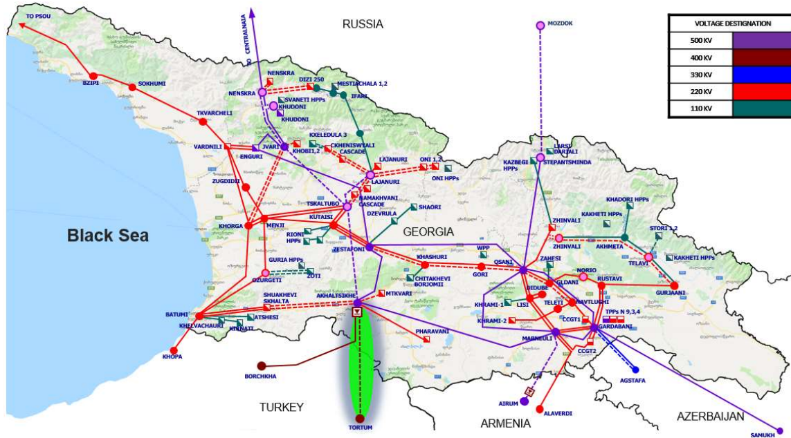
Fig. 3.11 Single-line diagram of "Akhalsikhe-Tortum" Project
