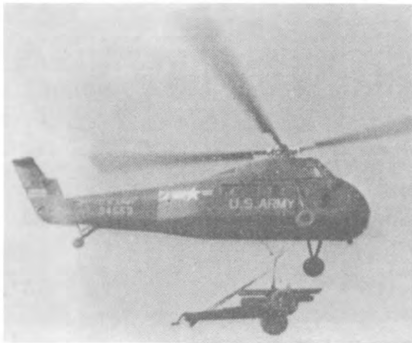
EARLY MOVEMENT OF ARTILLERY BY AIR. CH-34 with 105-mm. carriage.
