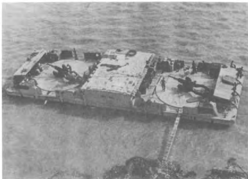
RIVERINE PLATOON MOORED TO CANAL BANK. Living quarters are located in center, ammunition storage on each end.
