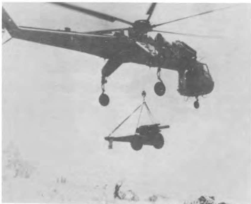
CH-54 LIFTING 155-MM. HOWITZER
