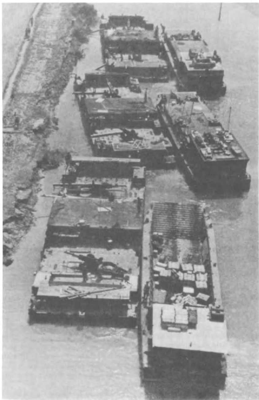
RIVERINE BATTERY POSITION. Six M102 howitzers preparing for an operation (fire direction center located in center right barge).
