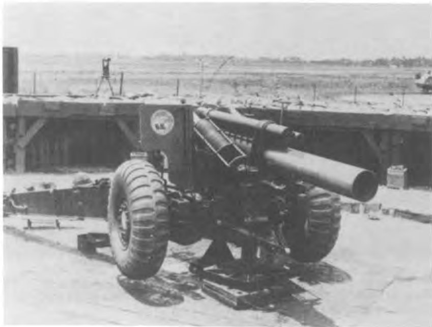
155-MM. HOWITZER POSITION USING SPEEDJACK AND COLLIMATOR. Speedjack is under center of howitzer, collimator to the rear of howitzer on sandbags.
