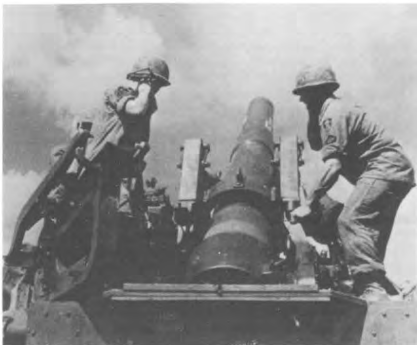
FIELD FORCE ARTILLERY. Eight-inch howitzer ready to fire (note gunner's quadrant held by man on left).
