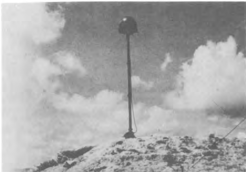
TPS-25 GROUND SURVEILLANCE RADAR
