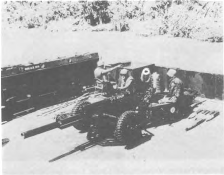
RIVERINE GUN SECTION IN TRAVELING CONFIGURATION. Note the five Beehive rounds at left of trails.
