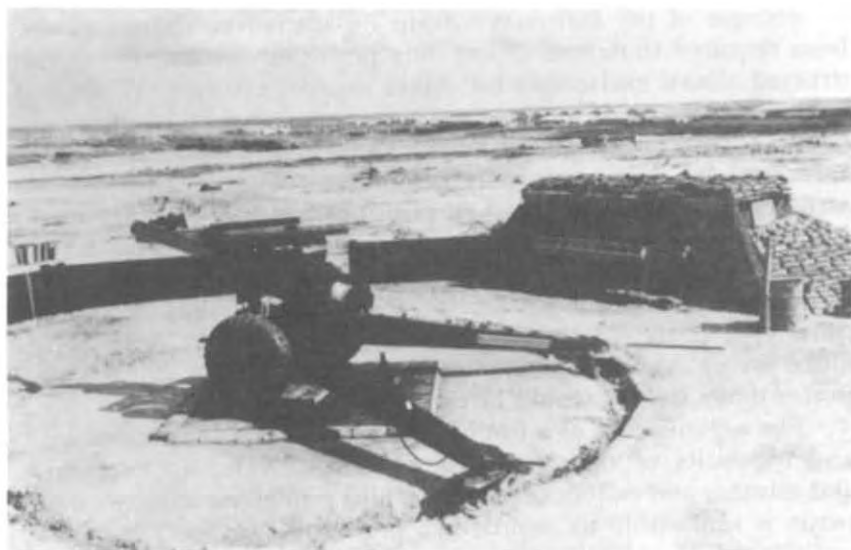
TYPICAL TOWED 155-MM. POSITION. Note trail blocks.
