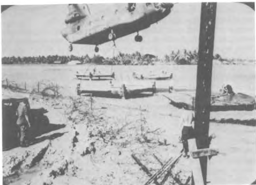
CH-47 EMPLACING AIRMOBILE FIRING PLATFORM
