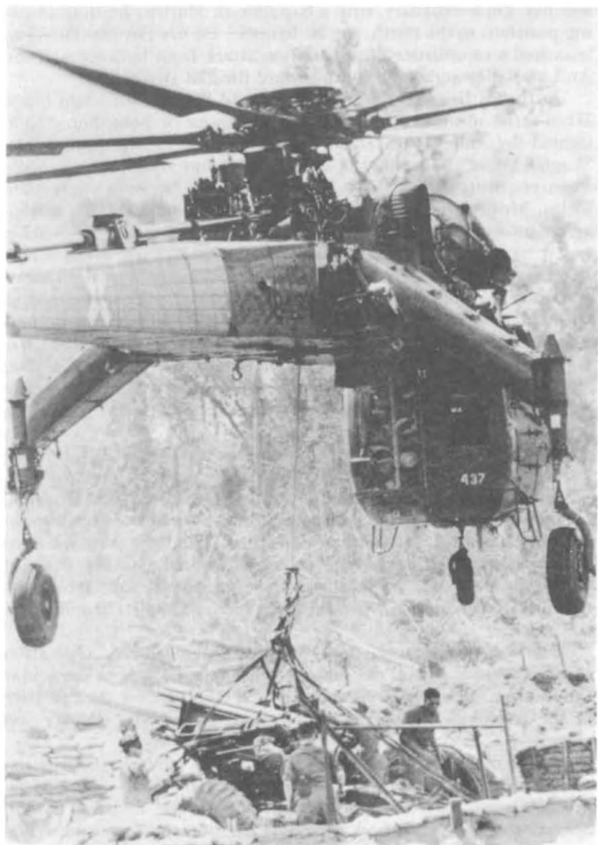
CH-54 EEMPLACING 155-MM. HOWITZER
