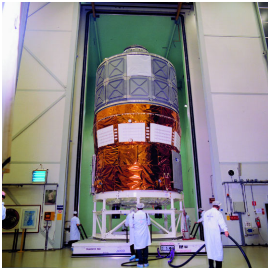
ATV STM testing at ESTEC. Above: in the Large European Acoustic Facility. Facing page: with (from left) Director General Antonio Rodotà, Head of MSM Manned Spaceflight Programme Department Alan Thirkettle, Mr. Feustel-Büechl, ESA Director of Administration Daniel Sacotte and ATV engineer Geoffrey Beckwith.
