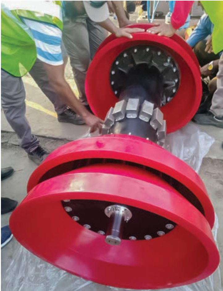
On stream pigging of 30" X 84 k.m. Hatikumrul-Bheramara pipeline of GTCL
