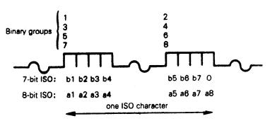
Fig. 3 Use of Binary Groups of the Time-and-Control Code to Describe the ISO Character Coded with 7 or 8 Bits
