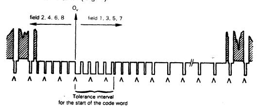
Fig. 5 Start of the Code Word in the Field-Blanking Interval (625/50)
