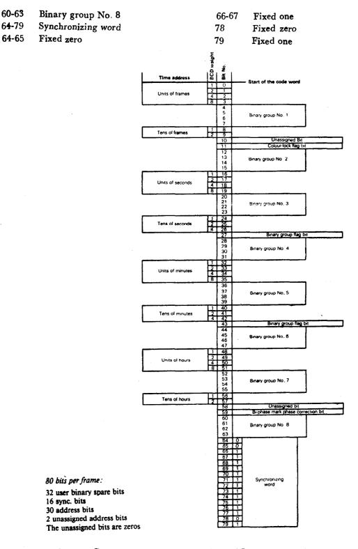
Fig. 2 Constitution of the Code Word (Longitudinal Code)
