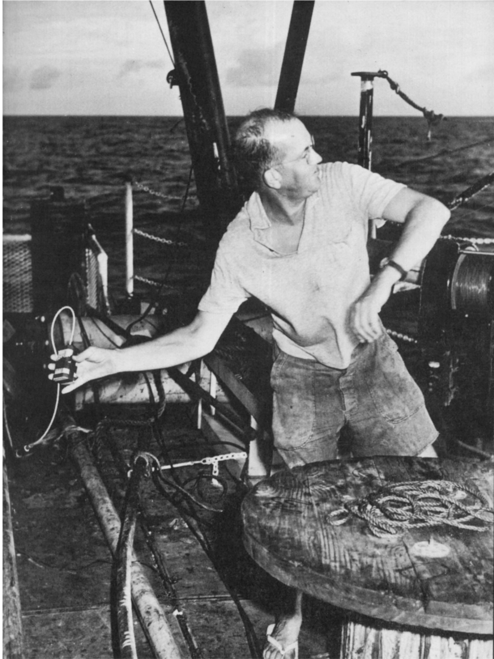
Russell W. Raitt throwing a one-half-pound TNT charge from the Spencer F. Baird , Capricorn Expedition, 1952.
