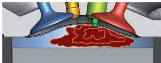
Fig. 1: Illustration of the flame propagation within an internal combustion engine leading to FWI.
