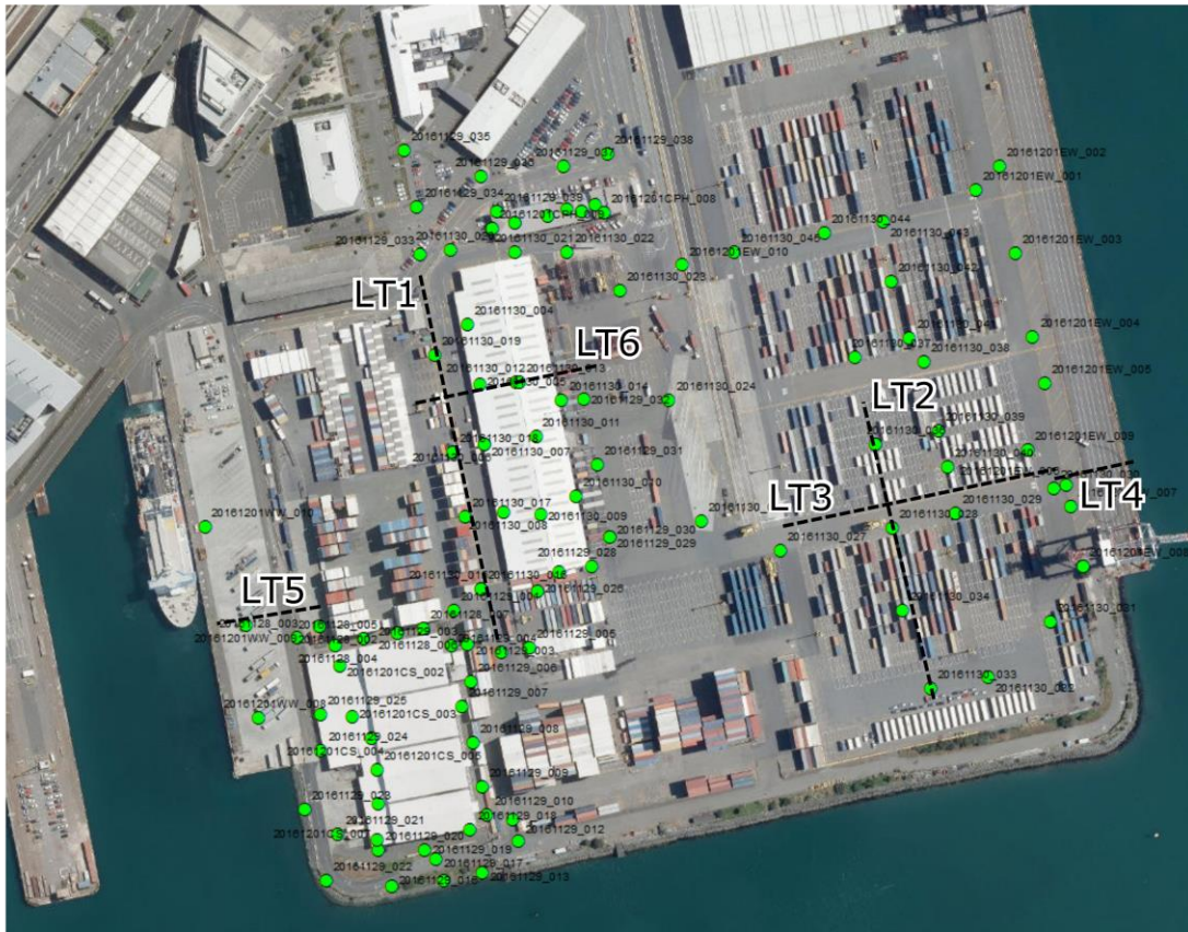
Figure 16: Locations (green circles) where ground-based LiDAR scans were obtained at the CentrePort. Additional scans were captured inside the Cruise Ship Terminal to the North that are not shown. Transects from the LiDAR data shown later in the report are identified. Note that the basemap is from ESRI prior to the earthquake.
