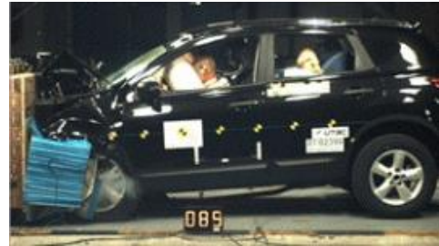
Offset crash test at 64km/hr
