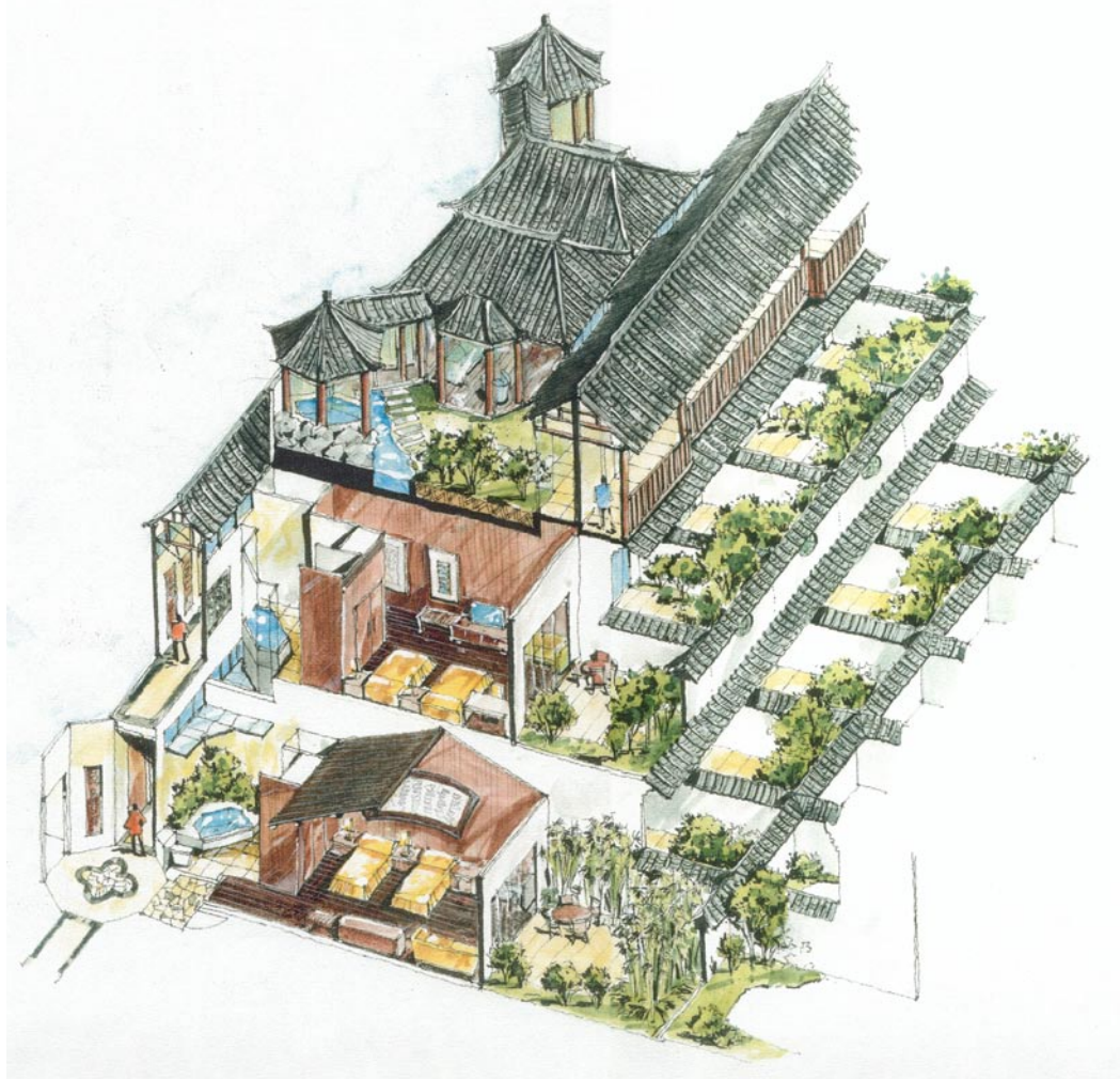
Fig 1. Rooms stacked to create terraces
