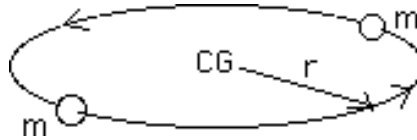
Fig. 3 - Two masses orbiting around their common center of gravity
