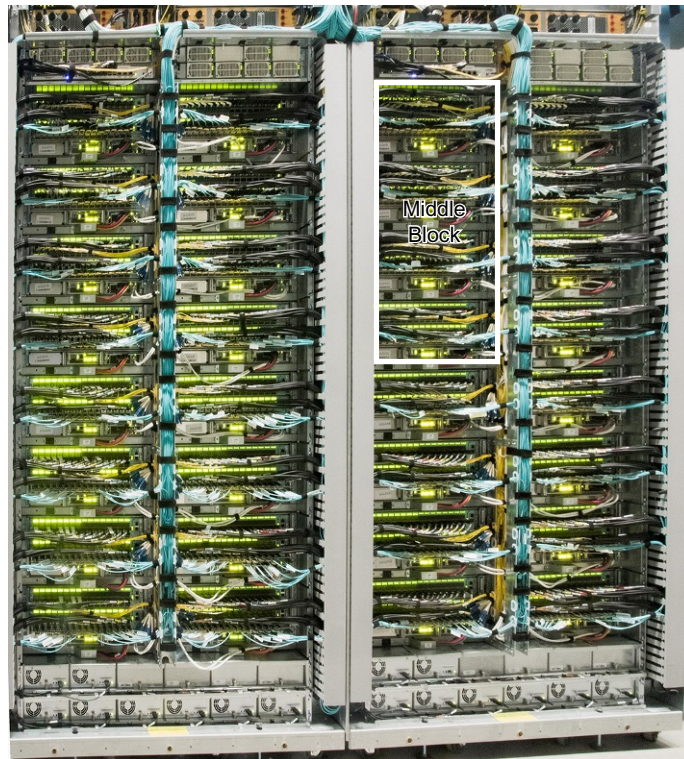
Figure 6.33 Middle blocks of the Jupiter switches housed in racks. Four are packed in a rack. A rack can hold two spine blocks.
