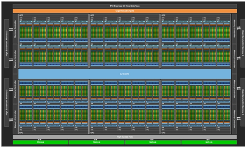
Figure 4.15 Full-chip block diagram of the Pascal P100 GPU. It has 56 multithreaded SIMD Processors, each with an L1 cache and local memory, 32 L2 units, and a memory-bus width of 4096 data wires. (It has 60 blocks, with four spares to improve yield.) The P100 has 4 HBM2 ports supporting up to 16 GB of capacity. It contains 15.4 billion transistors.
