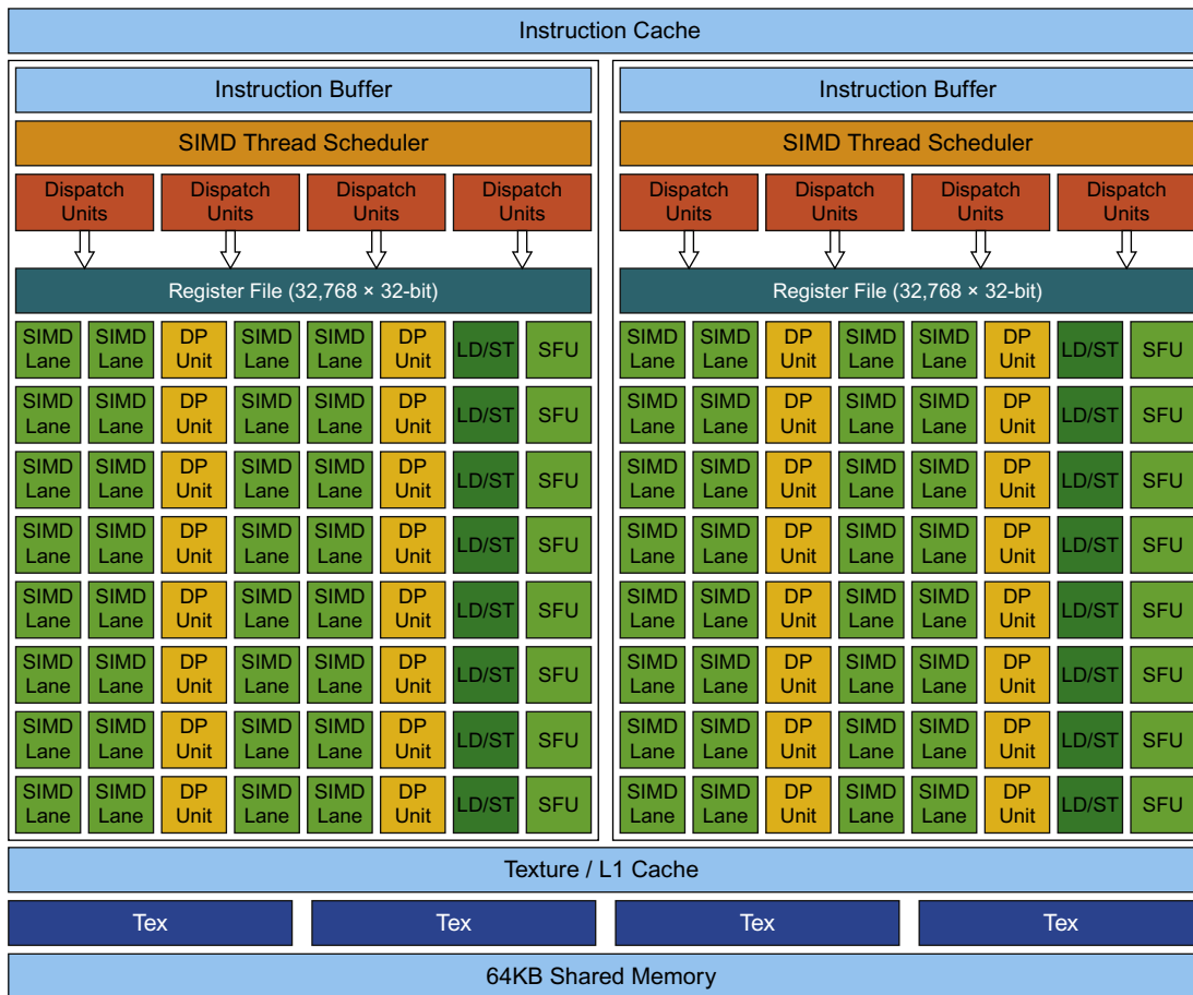
Figure 4.20 Block diagram of the multithreaded SIMD Processor of a Pascal GPU. Each of the 64 SIMD Lanes (cores) has a pipelined floating-point unit, a pipelined integer unit, some logic for dispatching instructions and operands to these units, and a queue for holding results. The 64 SIMD Lanes interact with 32 double-precision ALUs (DP units) that perform 64-bit floating-point arithmetic, 16 load-store units (LD/STs), and 16 special function units (SFUs) that calculate functions such as square roots, reciprocals, sines, and cosines.
