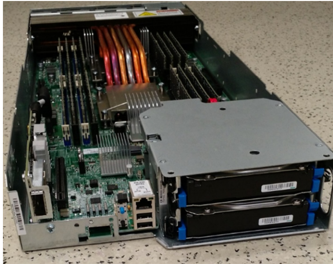
Figure 6.34 An example server from a Google WSC. The Haswell CPUs (2 sockets \times 18 cores \times 2 threads = 72 “virtual cores” per machine) have 2.5 MiB last level cache per core or 45 MiB using DDR3-1600. They use the Wellsburg Platform Controller Hub and have a TFP of 150 W.
