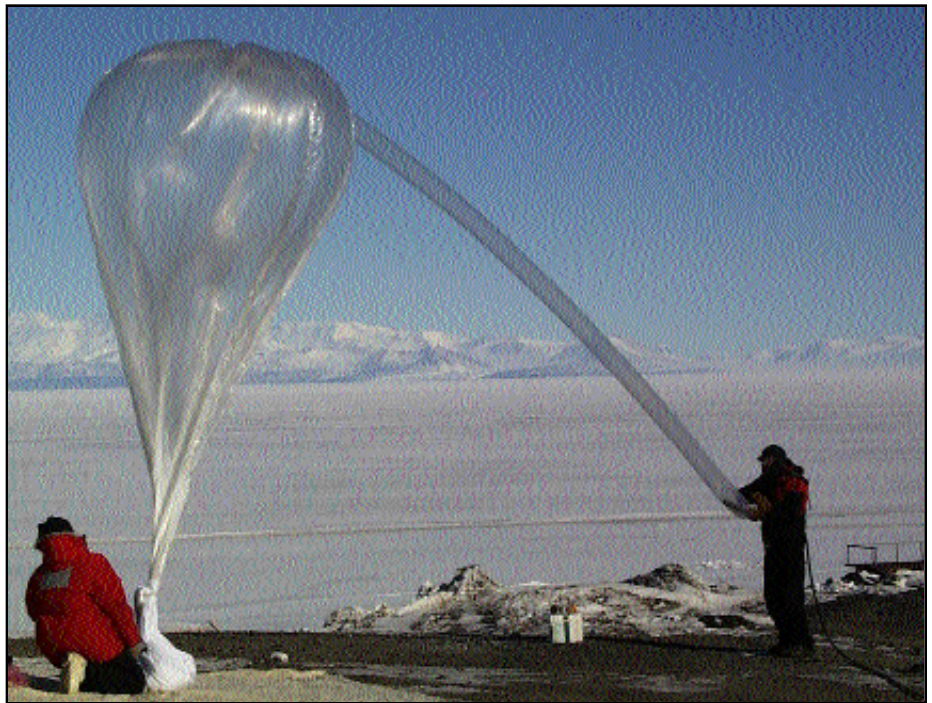
Liz Sinclair and Donal Lukens, lab technicians on a University of Wyoming research team, launch one of their last balloon-borne experiments of the season from the VXE-6 platform. The balloon and accompanying ozone sonde were sent up to 32 kilometers to study levels of ozone in the stratosphere.
