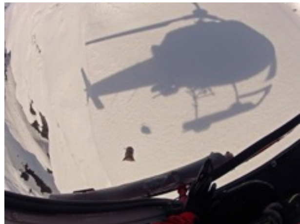
One of our standard burlap-bagged 12.5 kg ANFO charge, with 2m double cap and fuse, drops from the helicopter.
