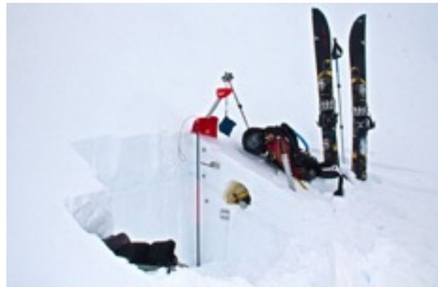
Snowpit for field snow studies, with snow profile, temperature, and density set up for measurement.
