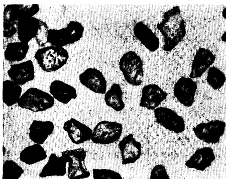
Photomicrograph of silica sand produced from Potsdam sandstone, showing quartz grain shapes in screen fraction -100+150 mesh. ( \times 35 .)
