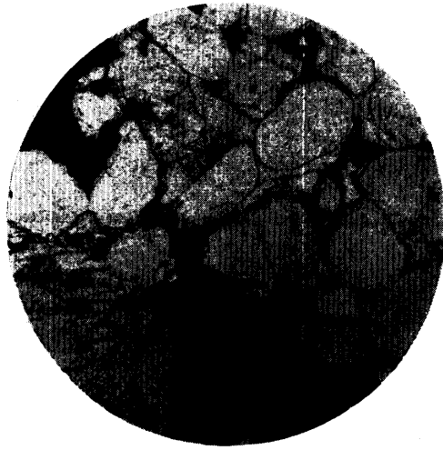
Photomicrograph of a section of drill core from the quarry of Kingston Silica Mines, showing sandstone containing intergranular pyrite (black). (X 35.)
