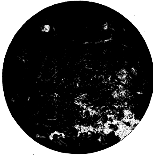
Photomicrograph of picrite-lamprophyre from an island in Leg lake. The bladed crystals are deep-brown biotite. The grains are olivine partially altered to light-green serpentine. ( \times 15 .)
