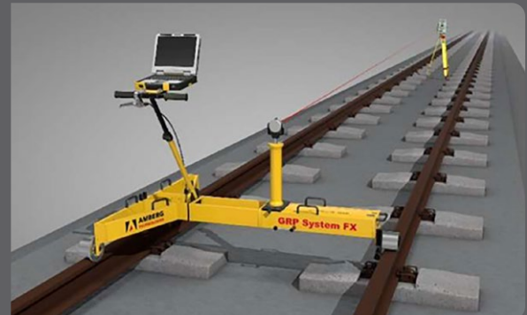
Rail survey trolley used to survey the track
