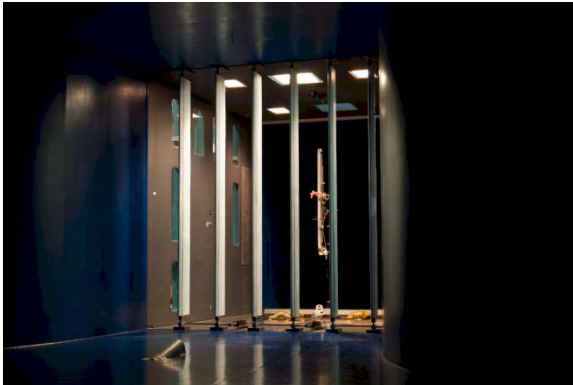
Figure 16: The Gust generator installed into the Wind Tunnel.
