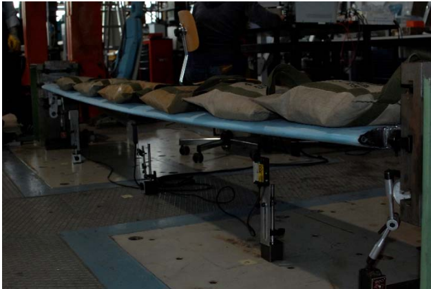
Figure 10: Static test on a single vane
