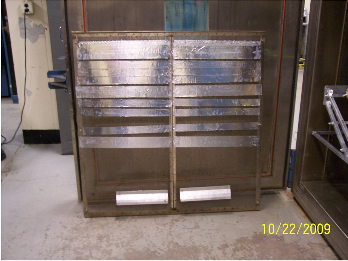
Figure 2-10. Airflow Redirection Solution
