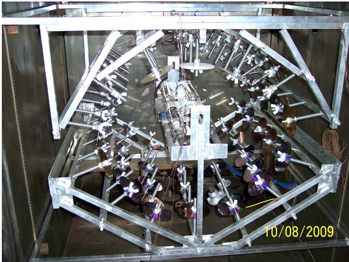
Figure 2-1. Disc Exposure Rack in Chamber
