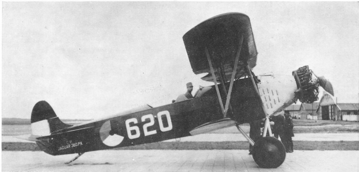
"Fokker C.VI" development of the basic C.V-D, powered by a 380-h.p. Jaguar engine. (Photo: Royal Netherlands Air Force)
