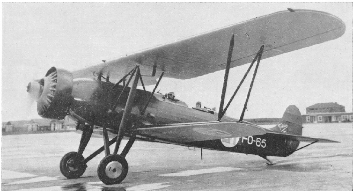
Finnish C.V-E equipped with 730-h.p. Bristol Pegasus. This is a Fokker-built machine; several of this version were built in Finland at the State Aircraft Factory at Tampere. (Photo: Fokker)
