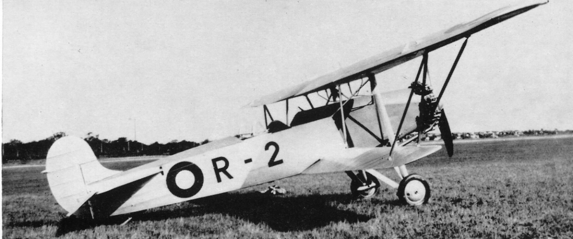
Danish C.V-E with Jupiter VI engine. The code R-2 appears to be a re-issue; the original R-2 was powered by a Lorraine Dietrich engine, and was a C.V-B of the first order batch.
