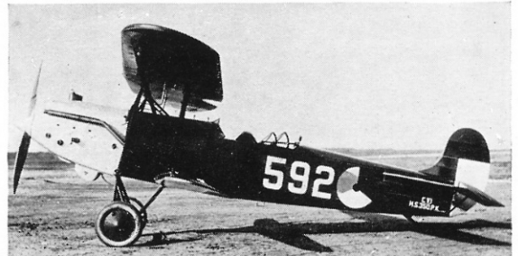
C.VI (C.V-D) operated by the Dutch Army Air Corps, with 350-h.p. Hispano-Suiza engine. The machine illustrated is the second in the original order batch. (Photo: Fokker)
