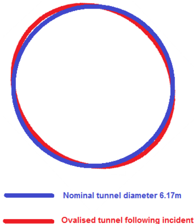
Figure 1 – Diagram of tunnel cross section showing ovalisation
