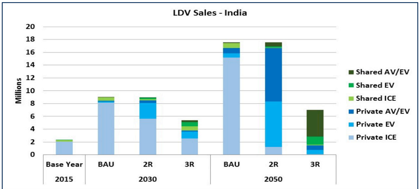
Figure 6a-b. Sales of private and shared vehicles for United States and India by scenario, year and vehicle type
