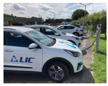
each with over 100km of range, on a typical winter's day. Smart controls ensured that the power was shared and could never exceed the capacity of the supply to site.
