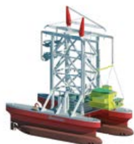
Decommissioning of top sides
