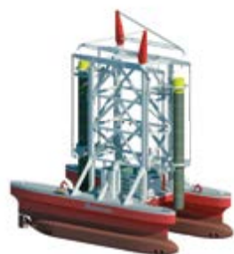
Wind Turbine Shuttle with two monopiles
