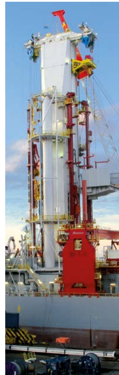
DMPT SIDE VIEW WITH RAISED CONSTRUCTION FLOOR
