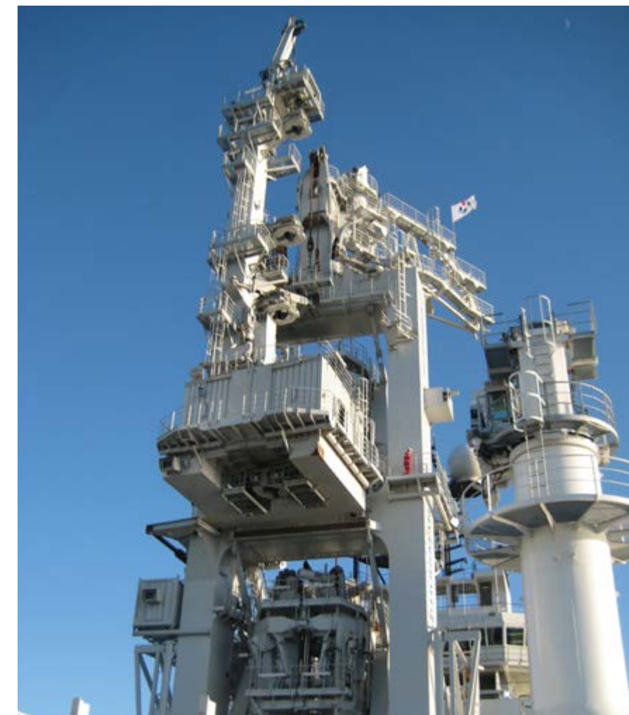
J-lay module with integrated welding station
