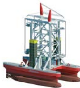
Wind Turbine Shuttle with piles
