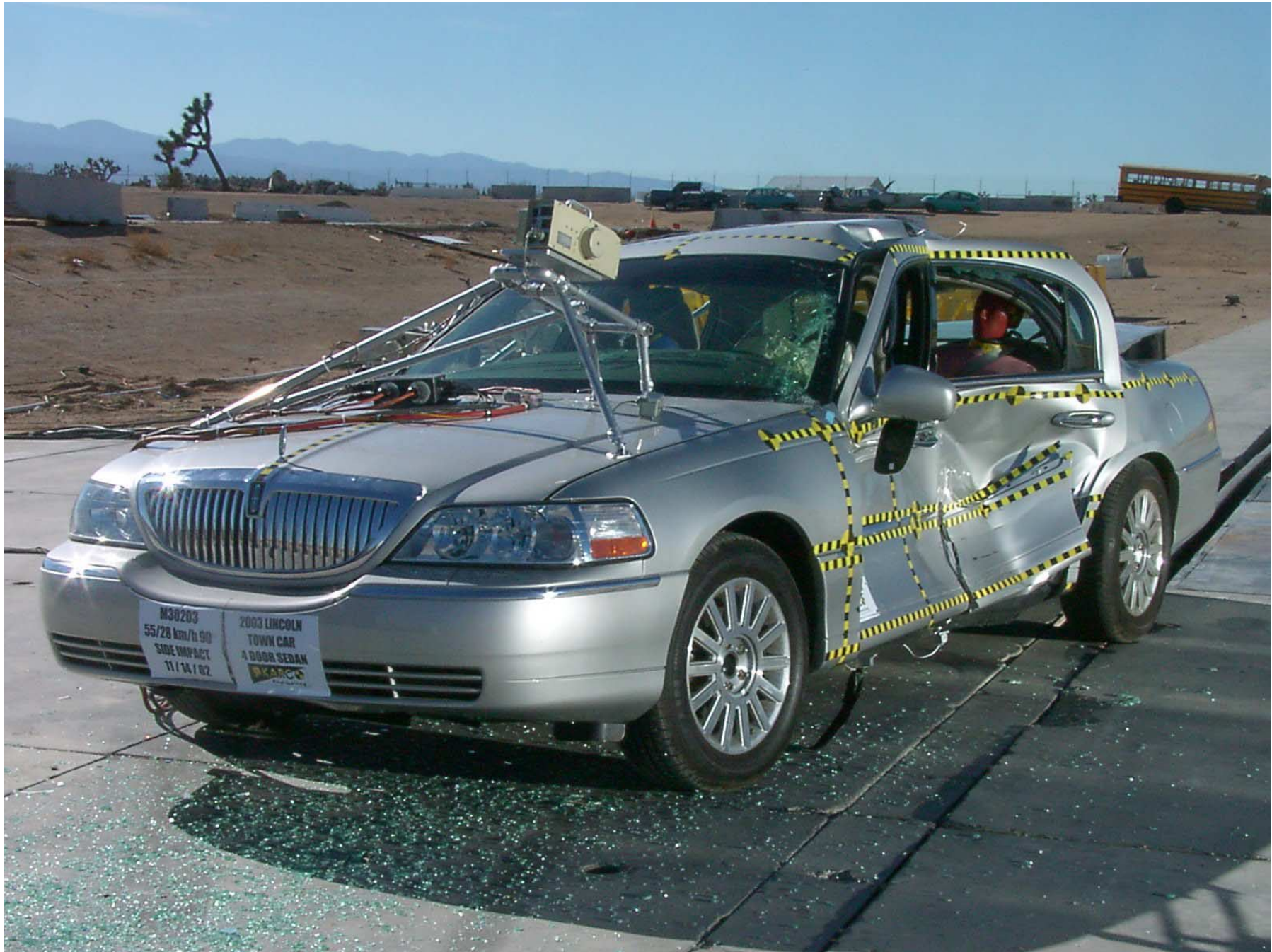
Figure A-8: Left Front \frac{3}{4} View, Post-Test (Trunk Lid Opened During Impact)
