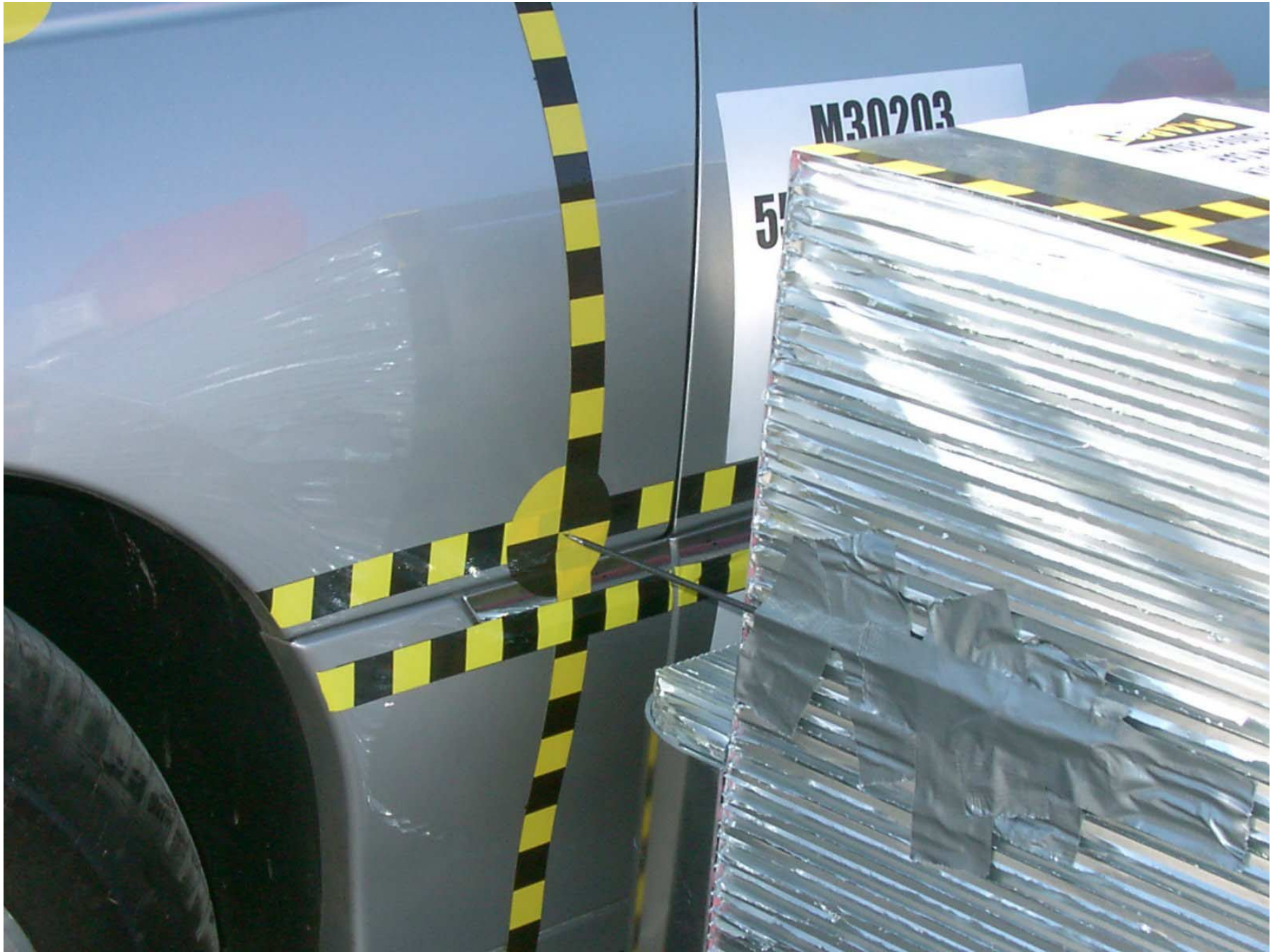
Figure A-19: Impact Point Target Set-up, Pre-Test
