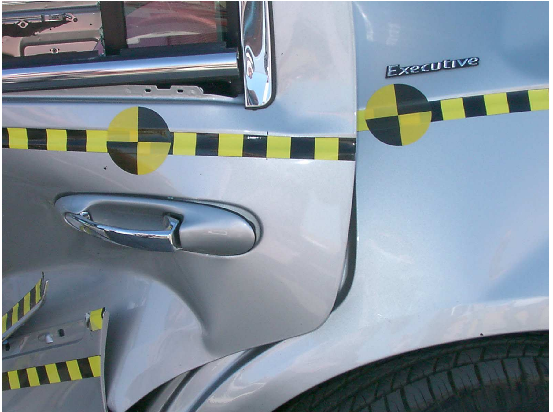
Figure A-28: Left Rear Door Closed, Post-Test
