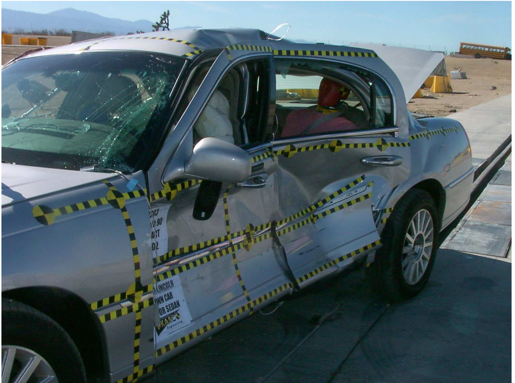
Figure A-22: Front ¾ View of Left Side Doors, Post-Test (Trunk Lid Opened During Impact)
