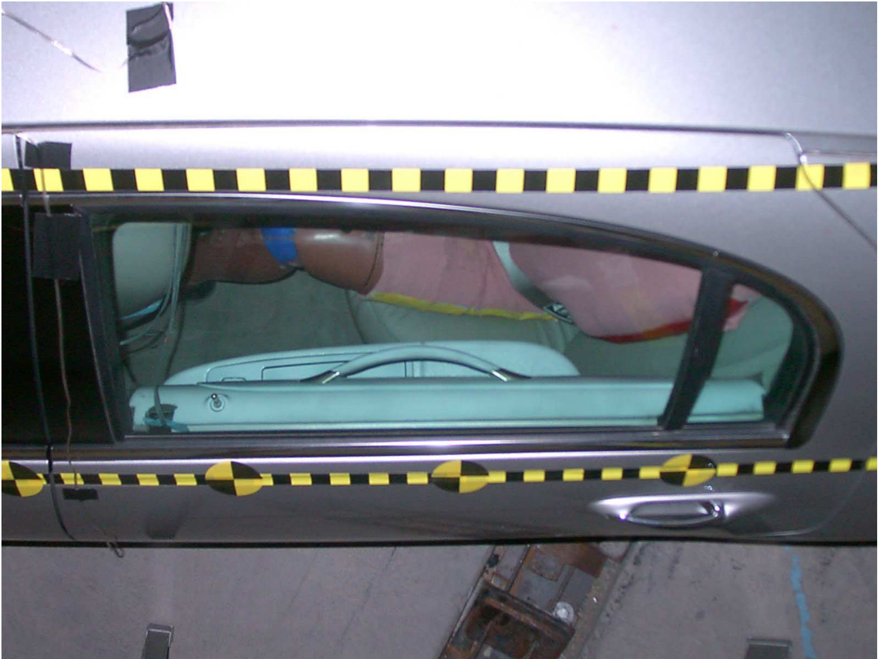
Figure A-41: Passenger Dummy Clearance, Pre-Test
