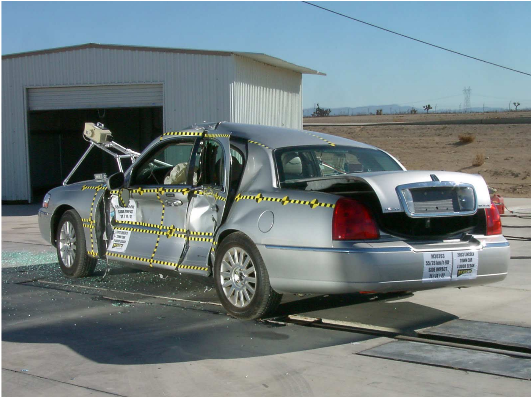
Figure A-12: Left Rear ¾ View, Post-Test (Trunk Lid Opened During Impact)
