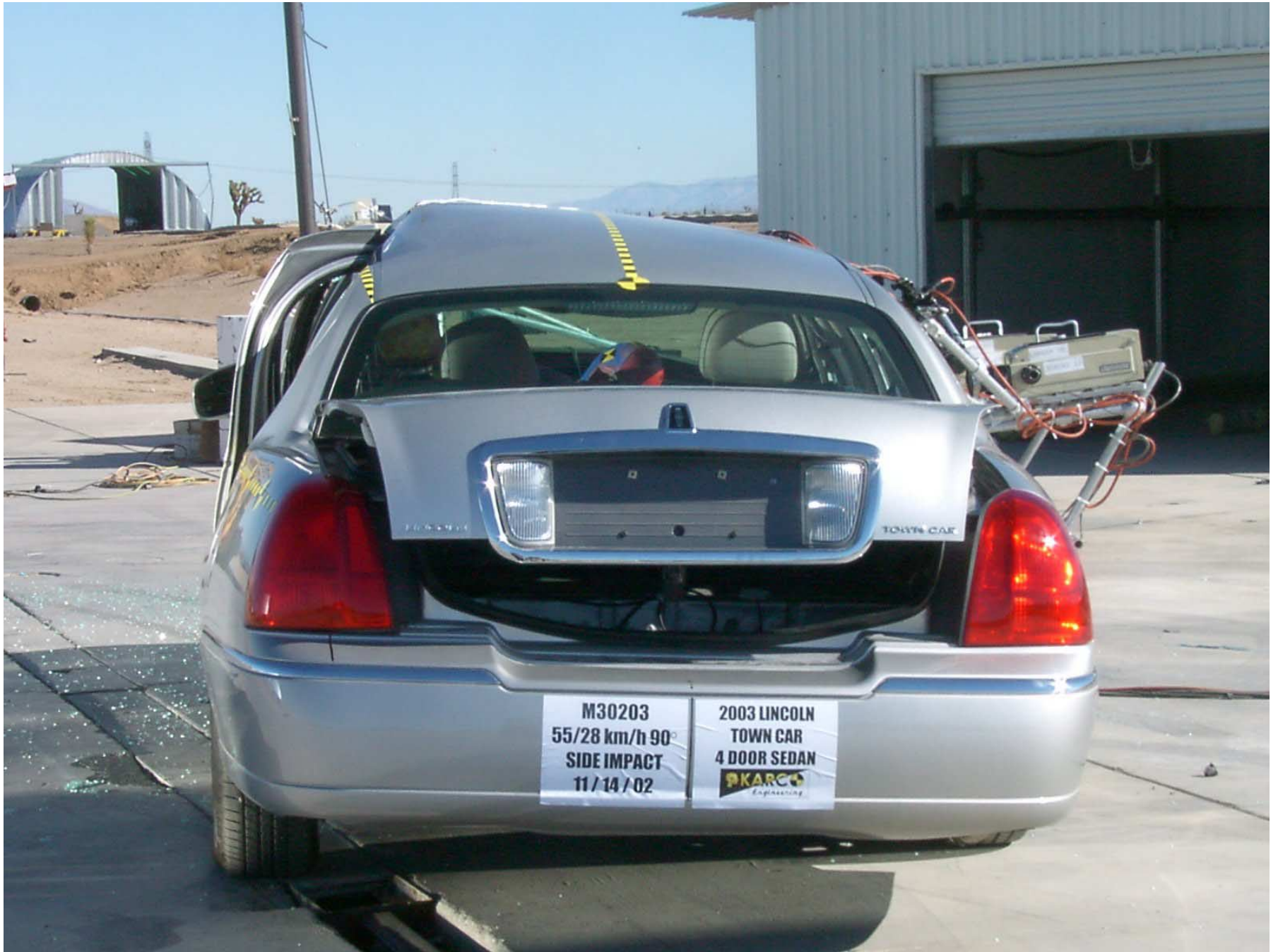
Figure A-14: Rear View, Post-Test (Trunk Lid Opened During Impact)
