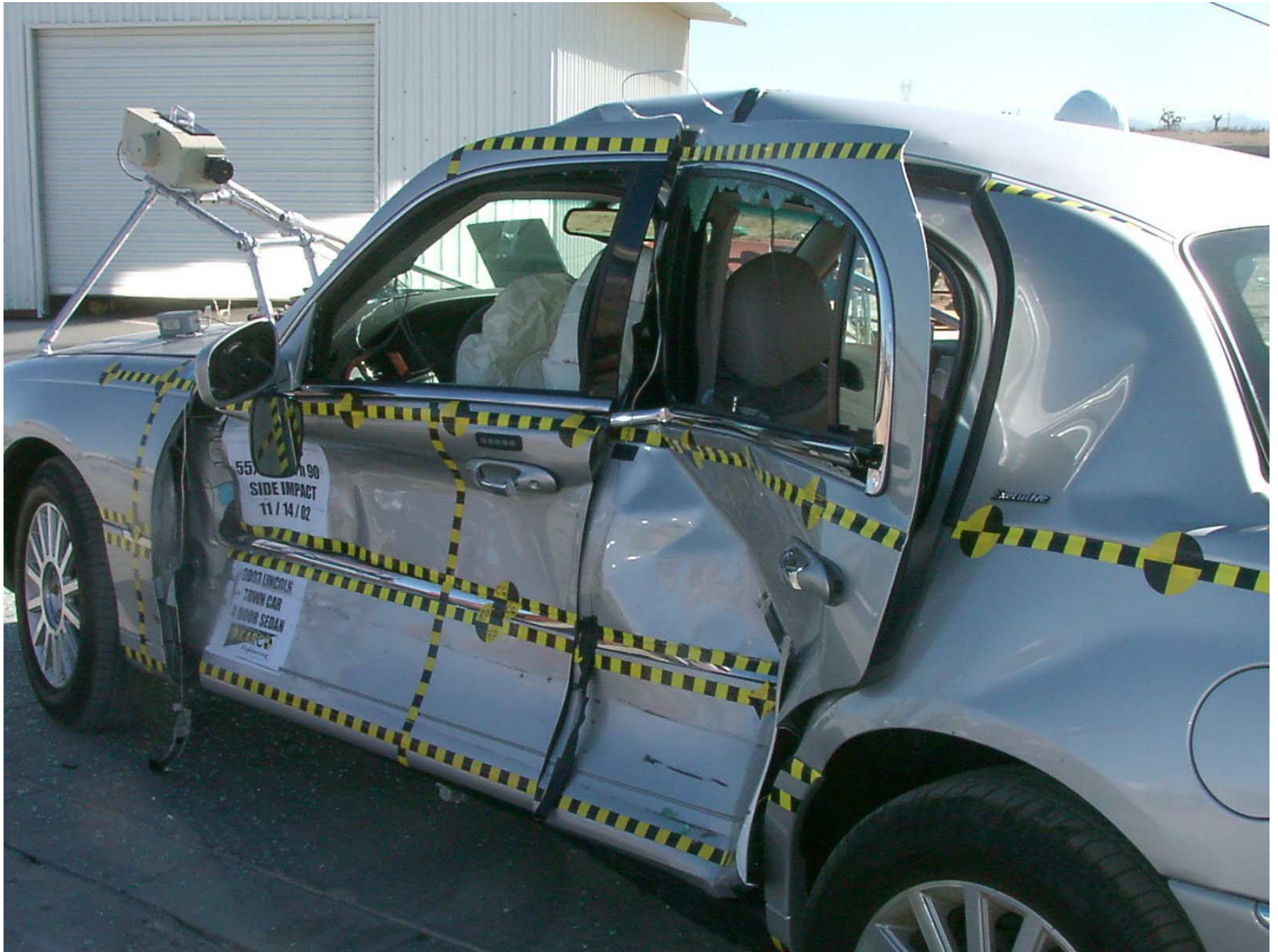
Figure A-24: Rear ¾ View of Left Side Doors, Post-Test
