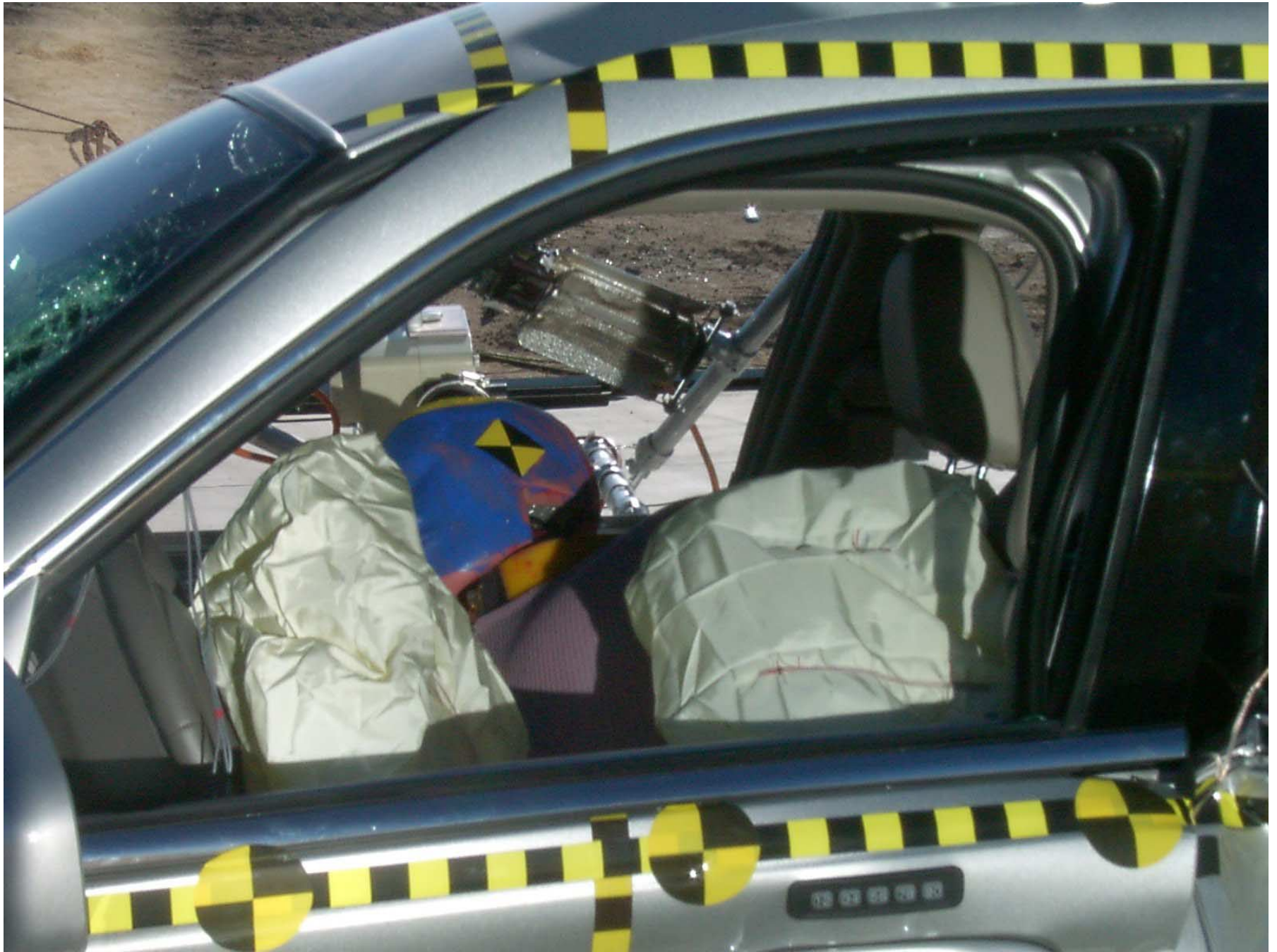
Figure A-31: Driver Dummy Left Side, Post-Test
