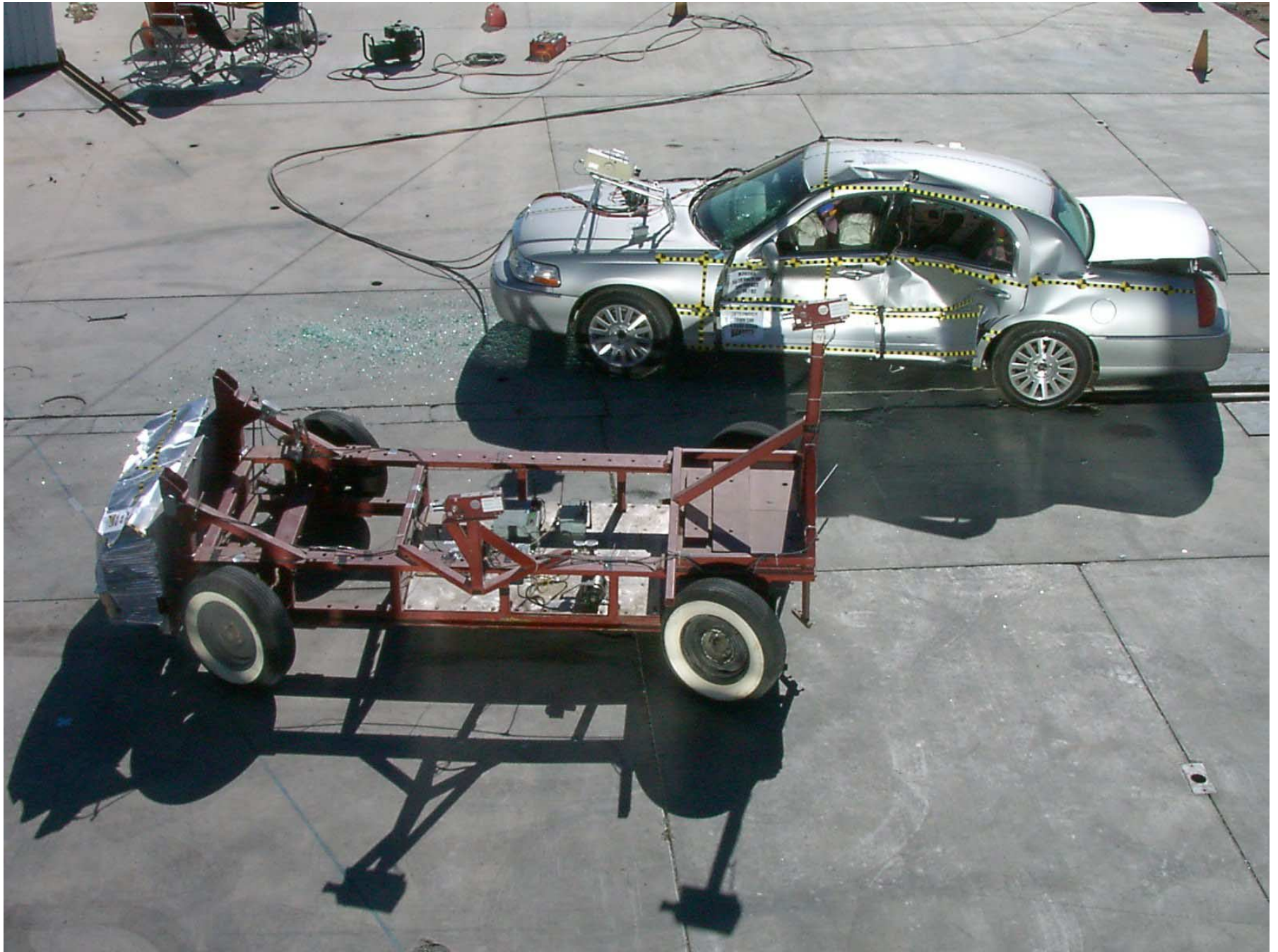
Figure A-16: Overhead Overall View, Post-Test (Trunk Lid Opened During Impact)
