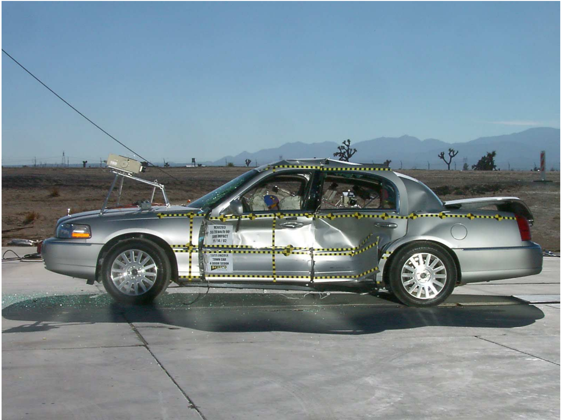
Figure A-10: Left (Impacted) Side View, Post-Test (Trunk Lid Opened During Impact)
