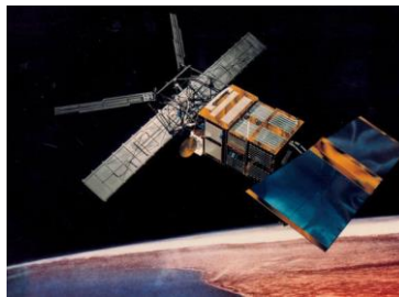
Fig. 9 Artist's illustration of ESA satellite ERS-2 [11]. High specular glints are expected to be caused by the reddish copper alloy protective foil
