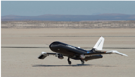
(b) NASA PTERA with Jetcat P200 engines
