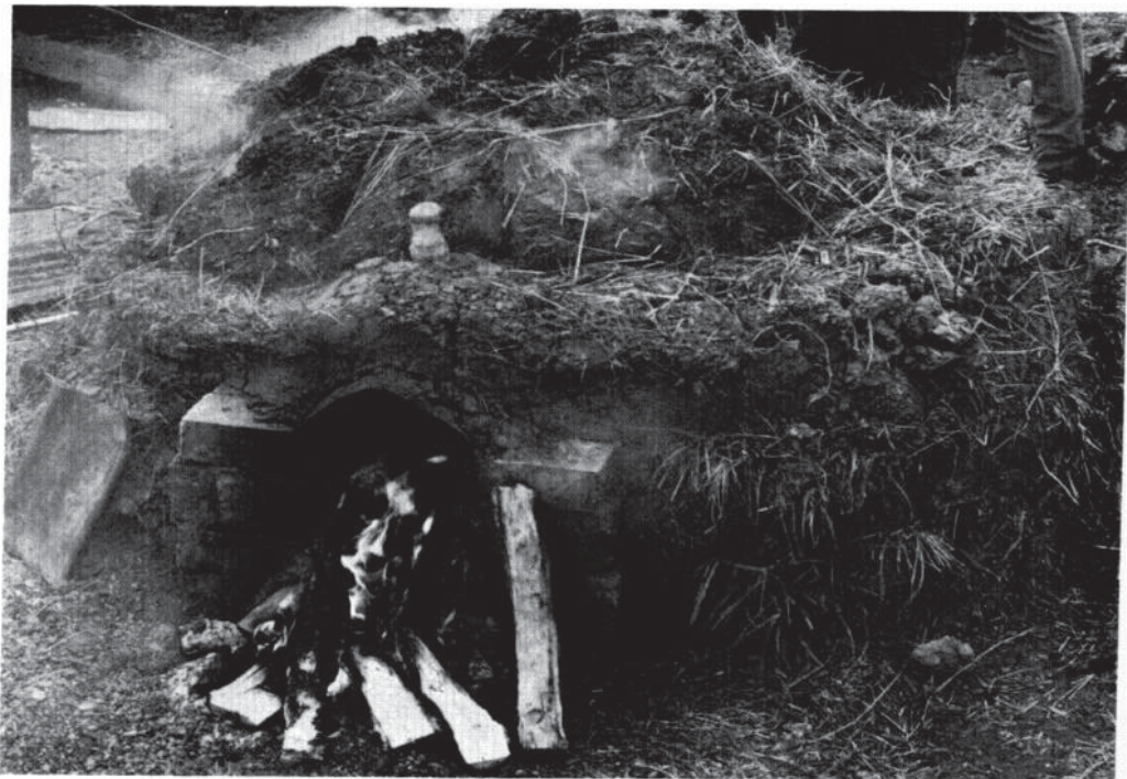
Barton-on-Humber, Kiln 6 towards the End of the Firing with Turf Dome covering the Load.
