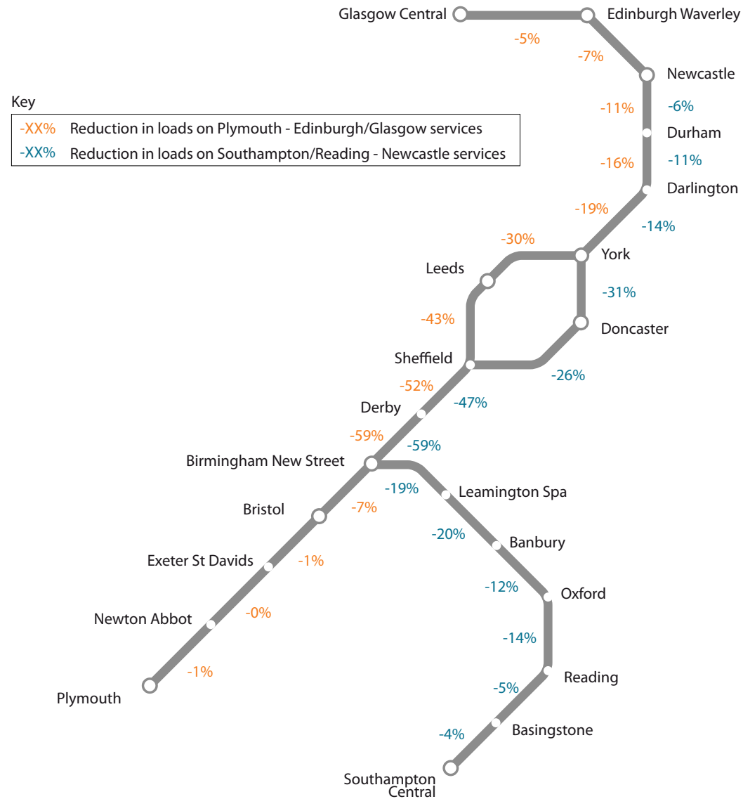
Figure A3.2 Reduction in loads on Plymouth to Edinburgh Waverley/ Glasgow Central and Southampton/Reading to Newcastle services as a result of HS2 Phase 2
