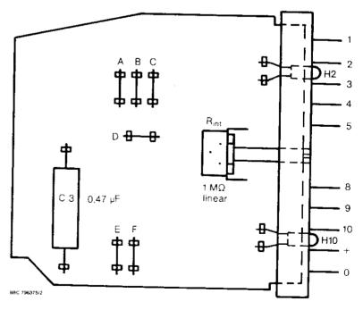
If other operating modes are desired then these can be realised by linking in accordance with the following plan.  $\frac{1}{2} \int_{\mathbb{R}^{n}} \frac{1}{2} \left( \frac{1}{2} \int$
