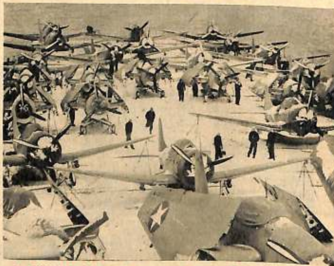
A SNOWY DAY on a carrier finds Dauntless dive bombers and Avenger torpedo planes covered in canvas and with wings to conserve valuable space.
