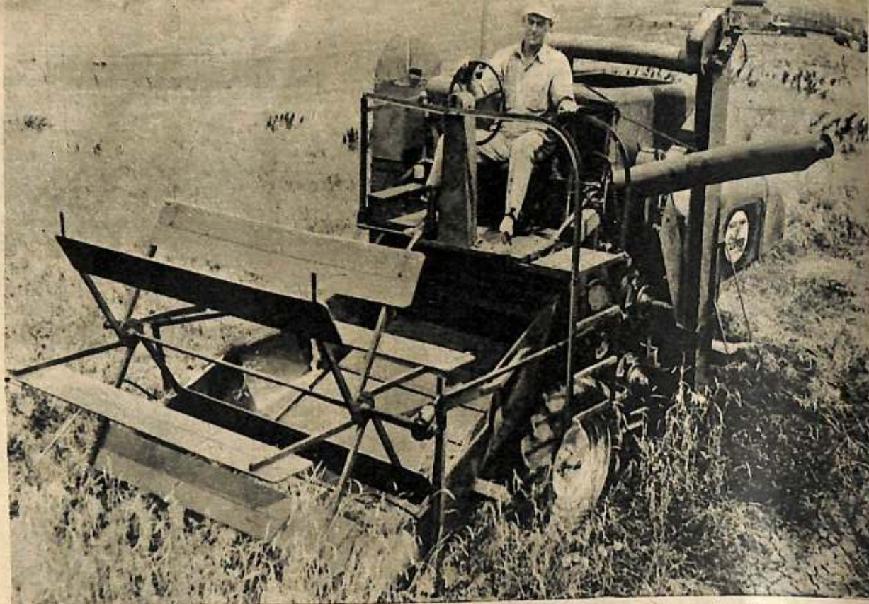
Does everything but light his cigarette for him. A one-man harvesting machine, with a pusher instead of a puller, threshes while it cuts and is especially designed for use on small farms.
