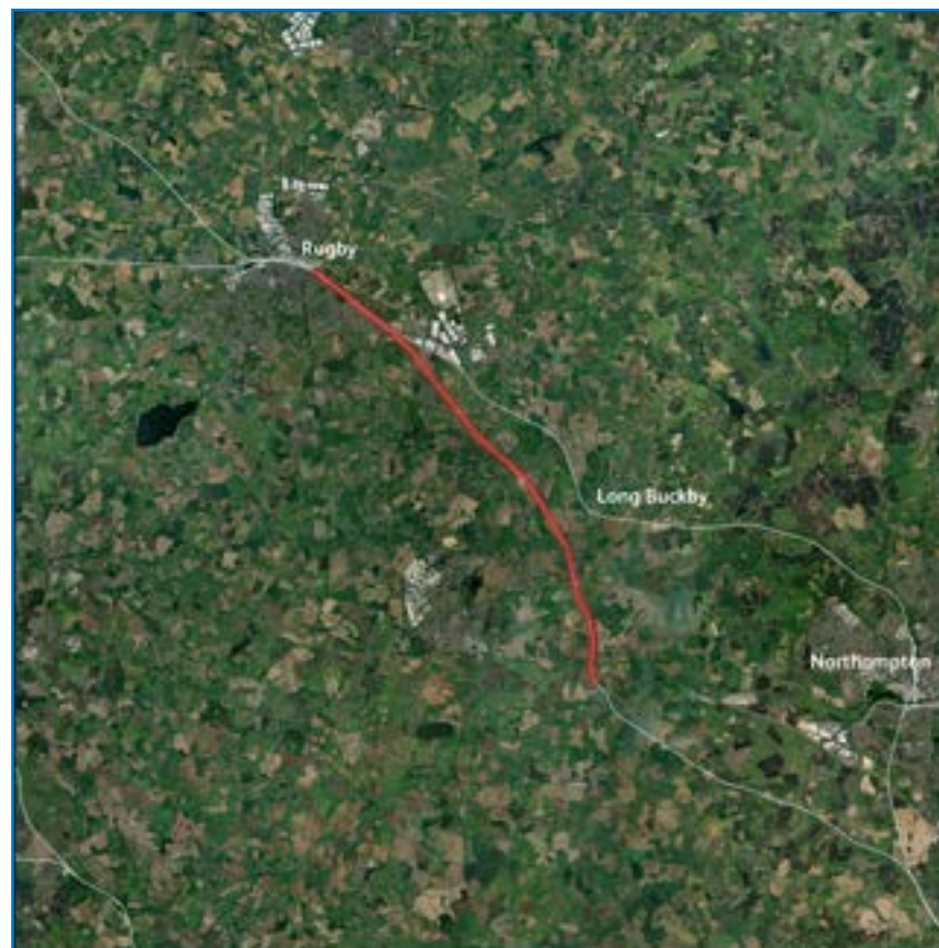
Figure 59: Scope area for fast line loops. Further work is required to determine the optimum position of loops in both directions, given the different results across freight and passenger-focused scenarios. Satellite imagery copyright ARCGIS, Esri, Maxar and Earthstar Geographics.
