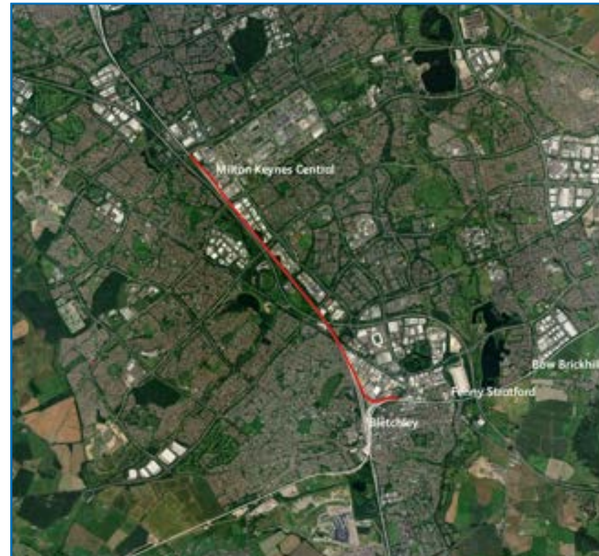
Figure 52: Scope area for highest priority infrastructure options identified as part of WCSSA, including Bletchley-Milton Keynes additional track and platforms, Milton Keynes Northern Connection and Bletchley Northeast Chord. Satellite imagery copyright ARCGIS, Esri, Maxar and Earthstar Geographics.
