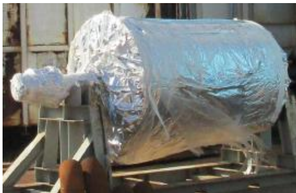
Figure 3-8 — GT 2-2 Compressor Rotor Storage and GT Housing Layup
