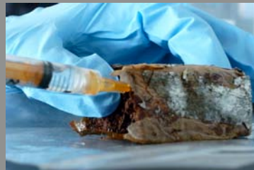
Injection of Paraloid B-72 consolidant
