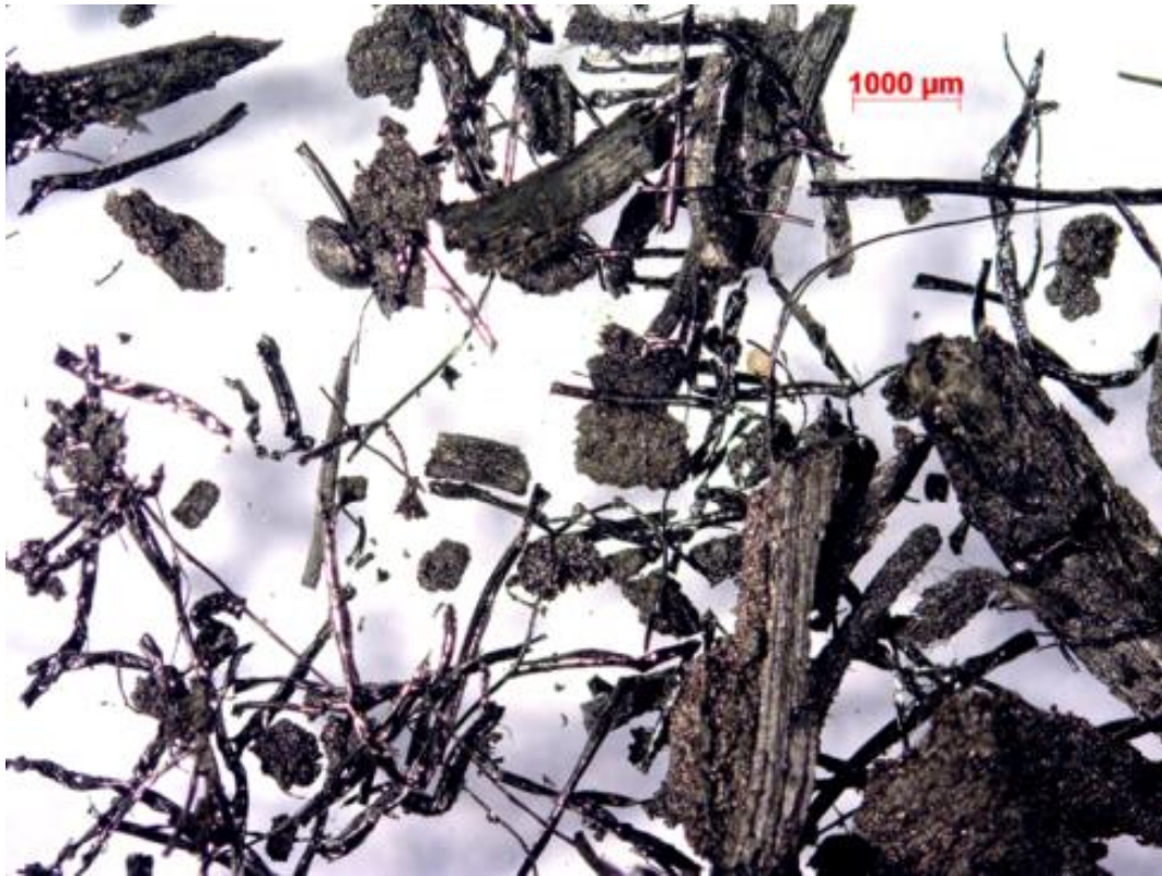
Figure 4.12: Optical microscope image of charcoalified Dicksonia antarctica stem material.
