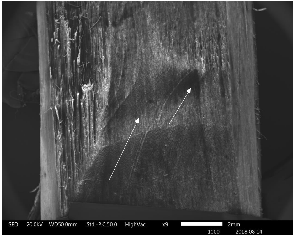
Figure 6.13 SEM photomicrograph showing slight tool marks and striations against the grain (arrows) visible on the dry specimen K1. Results shown are an example of similar observations across 8 separate replications.
