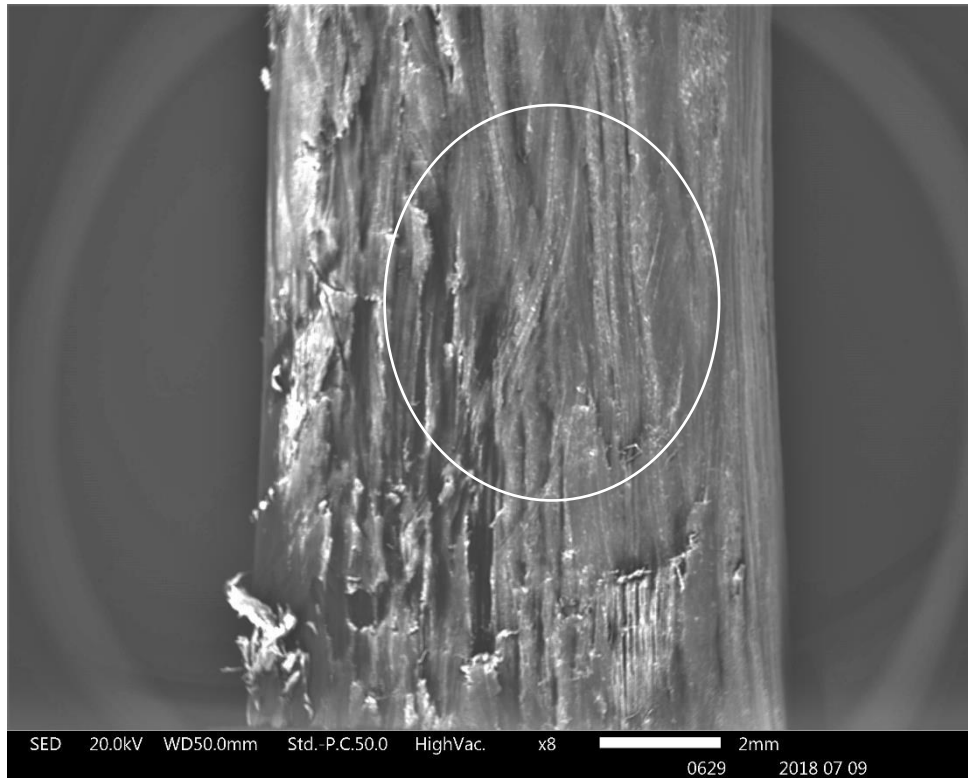
Figure 6.6 SEM photomicrograph of B2 showing the roughness of microfacets and striations that start to curve off to the side (circled). The micrograph is representative of observations from 8 separate replicates.
