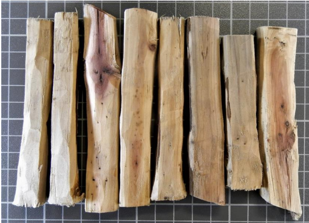
Figure 6.3b. Eight samples cut using a steel knife, K1-K8, left to right. K5-K8 were kept wet throughout the study and K1-K4 were allowed to dry before analysis.
