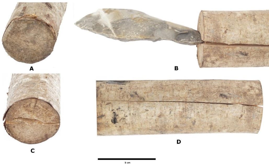
Figure 7.7 Hazel log splitting experiment using a biface wedge: A, before splitting; B, flint biface used as a wedge; C, D, basal and side splits resulting from the insertion of the biface wedge. (Scale = 5 cm.)
