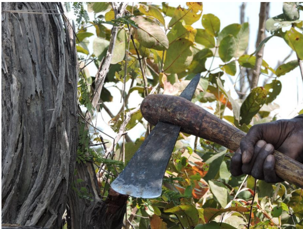
Figure 8.2. Hafted iron axe (socket arrangement) used to fell a medium size tree (10-12 m tall) Pericopsis angolensis ). The axe blade is 8 cm wide and Mr Mukopa's large axes have cutting edges that range from 6-8 cm in width.
