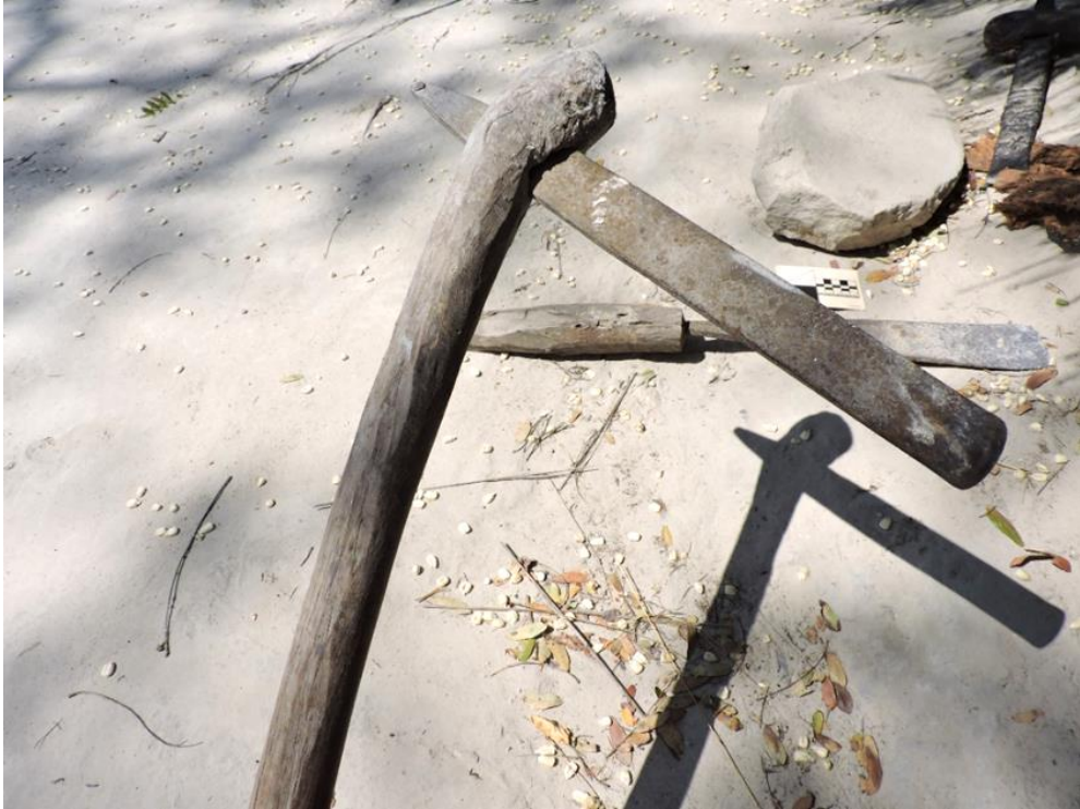
Figure 8.5. Long-bladed axe (foreground) and long-bladed chisel (background) for hollowing tree trunks. The quartzite block (rear, upper right) is a whetstone for sharpening axe and adze blades.
