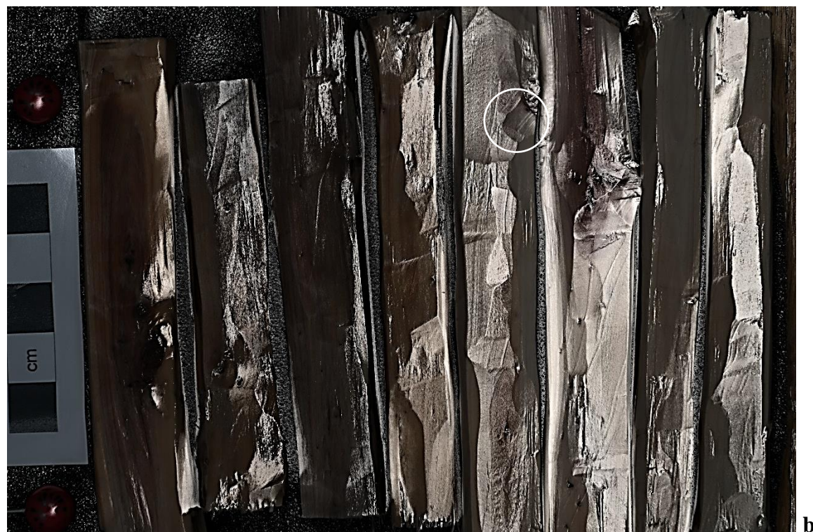
Figure 6.12 RTI images (a=diffuse grain view; b=spectral view) showing the smoothness of the facets and the presence of facet junctions on dry (K1-K4) and wet specimens (K5-K8) (white circles). Facets are less well-defined on wet specimens with marks on K8 losing the most definition. K1-K8, right to left.
