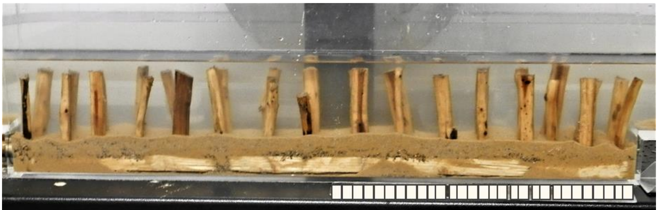
Figure 6.1. Photograph of wood samples in the flume inserted into a sand sediment base (Scale: 1cm per block).
