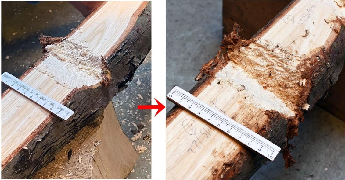
Figure 7.10. From left to right: gradual progression of cut during chopping.
