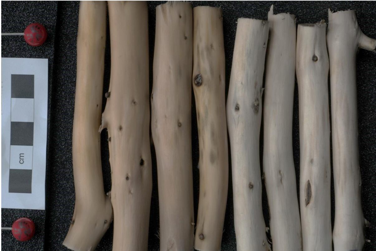
Figure 6.10 RTI image in normal viewing mode of the control sample (S1-S8, right to left) showing the smoothness of these specimens and the imperfections (knots) still visible.
