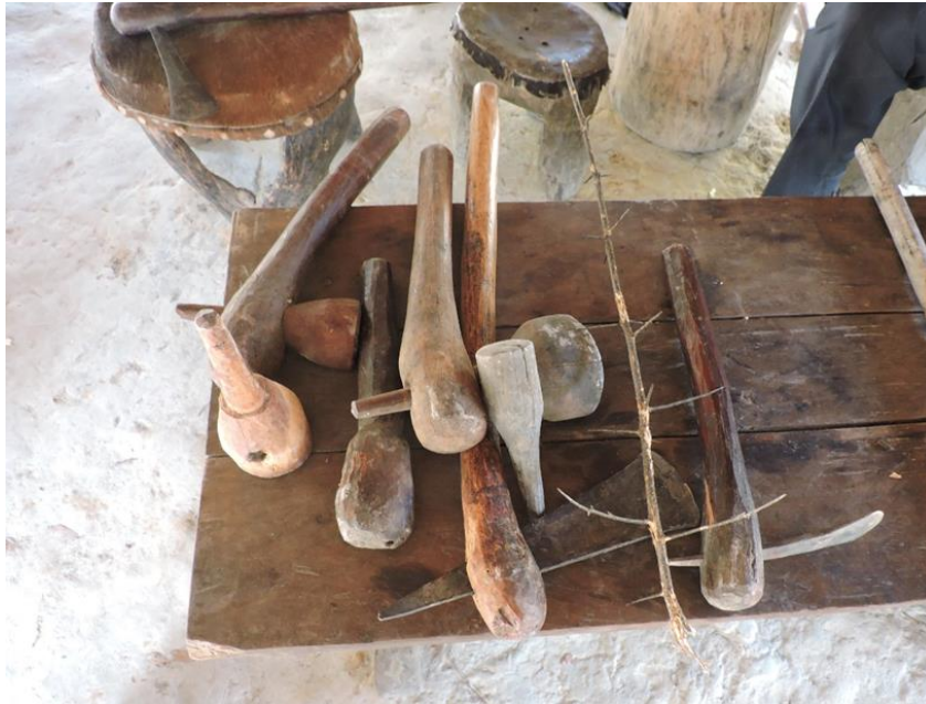
Figure 8.1. Tools made and used by Mr Mukopa. Adze (lower right), axe (lower central) and mallets (upper left). A loose mallet head is in the centre of the photo. The twig in the centre is a source of needles for sewing.
