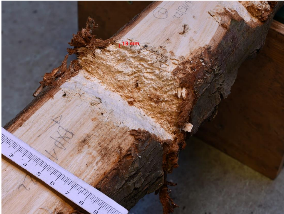
Figure 7.12. Stepwise incision, with indication of the depth (13 mm) of one of the first steps.
