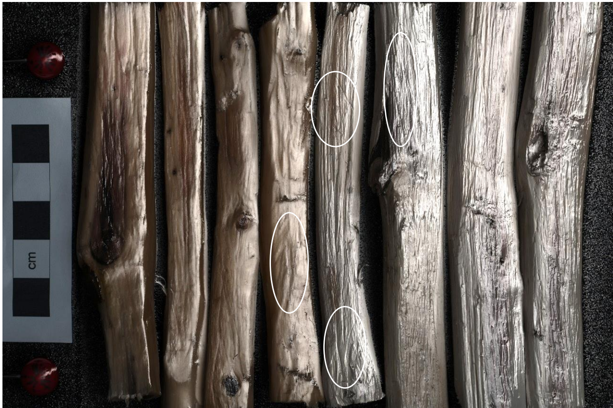
Figure 6.14 RTI images of bifacial tool shaping marks in normal (a) and spectral (b) viewing modes showing the smoothness of the facets on the wet specimens (B5-B8) compared with the dry specimens (B1-B4), but still maintaining facet junctions. White circles highlight a few striations that are still visible. B1-B8, right to left.
