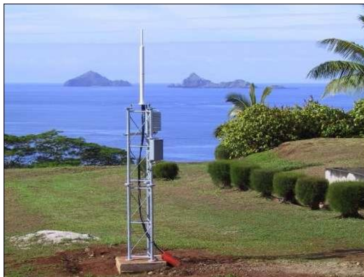
Figure 2.3.1: DORIS tracking station
