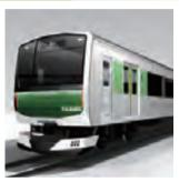
Catenary and battery-powered hybrid railcar train
