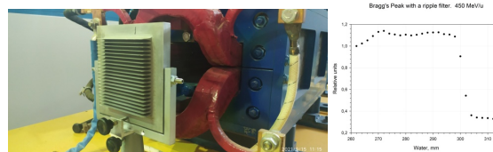
Figure 8: Aluminium ripple filter 16 mm on the left and Bragg's Peak on the right.
