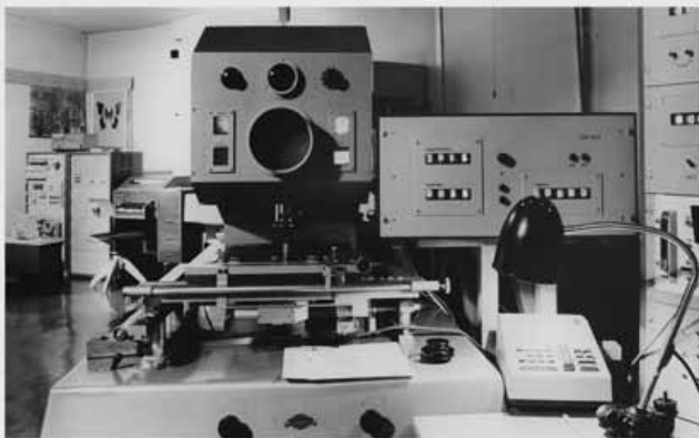
SARTORIUS iris diaphragm photometer, purchased in 1958; 1966 digital data printouts (punched tape); 1975 digital calibration; 1979 online connection to a KSR 4100 mini-computer
