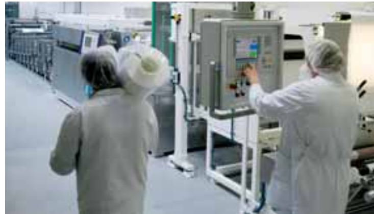
Second-generation casting machine based on the quenching method
