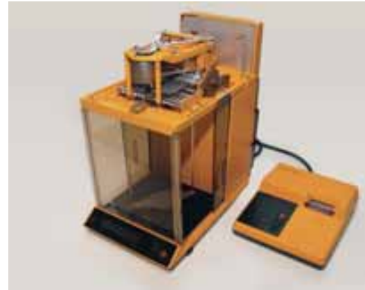
Electronic analytical balance, model 2003 MP1 (with the top cover lifted); year of manufacture: 1977; capacity: 160 g; readability: 0.01 mg
