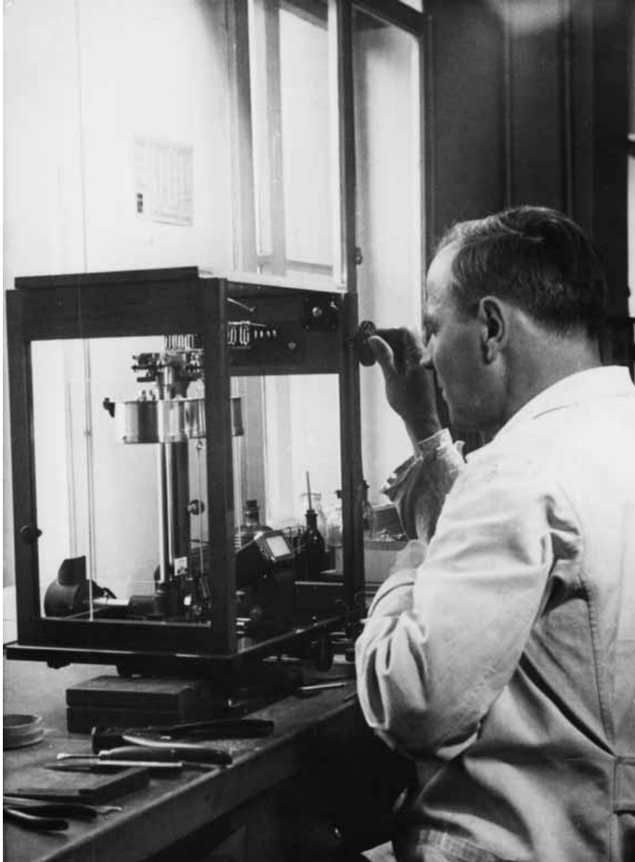
An employee performs calibration and adjustment on a model DP3 analytical balance.
