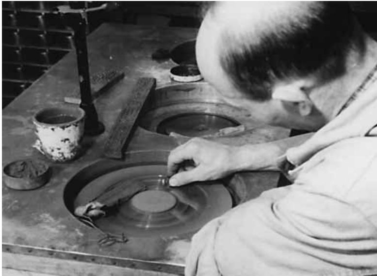
Polishing agate knife edges and bearings for balance beams
