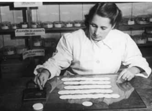
Visual inspection of membrane filter discs
