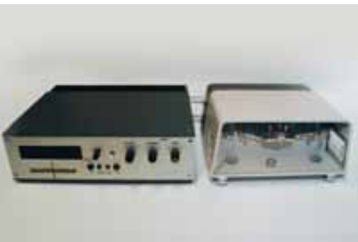
Electronic ultra-microbalance; year of manufacture: 1974; capacity: 3 g; readability: 0.3 \mu\text{g}
