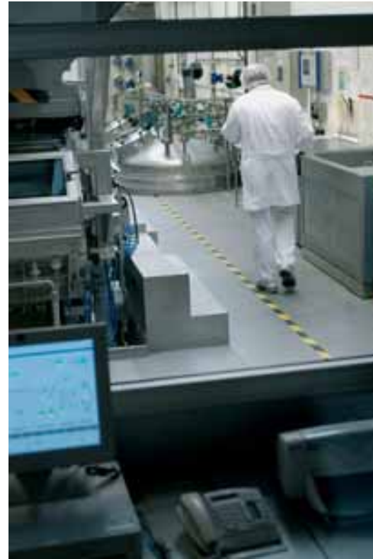
A view across the control station on a membrane casting machine and vats containing casting solutions.
