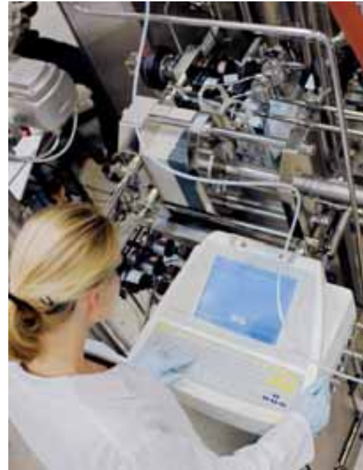
Integrity testing of filter systems using Sartocheck® 4
