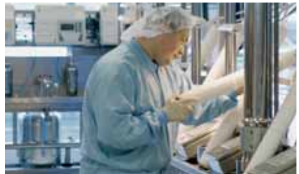
Individual testing of membrane filter cartridges
