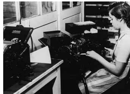
Before the introduction of EDP, records were produced using Ormig machines. This wet copying procedure was very time-consuming and unpopular due to the unpleasant odors it produced.
