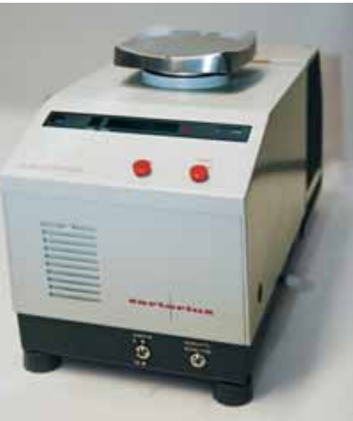
Electromechanical precision balance "Sartomat"; year of manufacture: 1978; capacity: 160 g; readability: 1 mg
