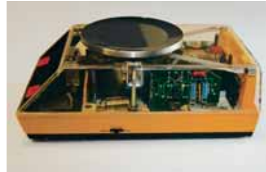
Precision balance 1264 004 (display model with plexiglass cover); year of manufacture: 1977; weighing capacity: 2,200 g; readability: 0.01 g
