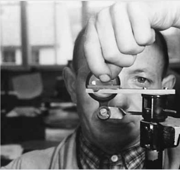
Attaching the reading scale
