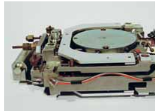
Weighing systems of electronic balances in conventional designs, 1975 – 1982
