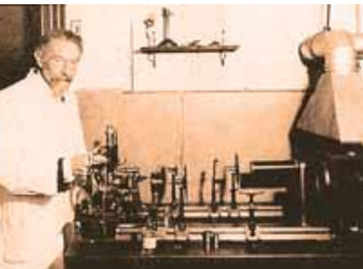
Prof. Richard Zsigmondy in front of an experimental setup for visualization of colloids under scattered light
