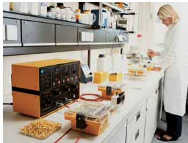
Testing the hybrid purity of seeds by phenotyping isoenzyme patterns obtained by electrophoresis using Sartorius cellulose acetate membranes
