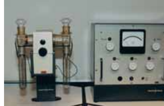
Vacuum ultra-microbalance; year of manufacture: 1962; weighing capacity: 3 g; readability: 0.1 µg
