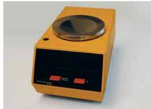
Precision balance, model 3713 MP; year of manufacture: 1977; capacity: 3,000 g/300 g; readability: 0.1 g/0.01 g
