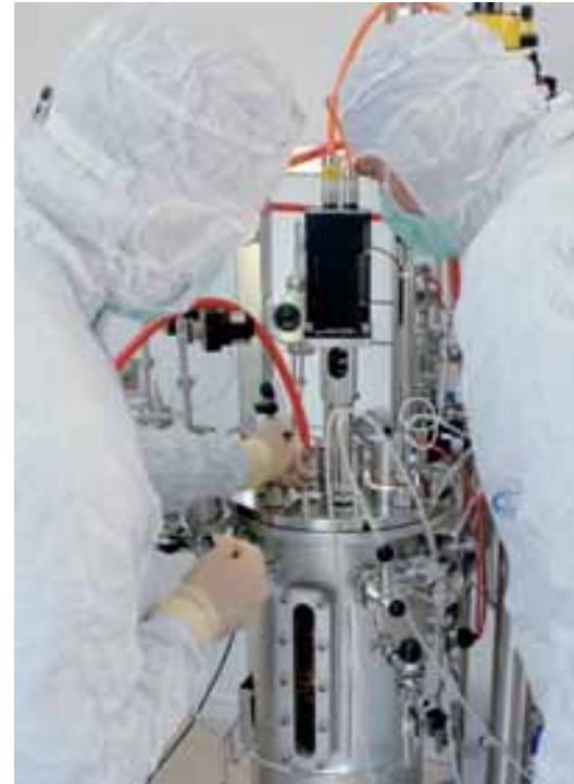
A BBI bioreactor is inoculated during the production of veterinary vaccines.
