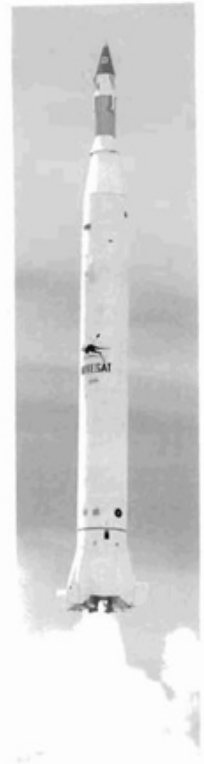
Figure 2 Launch of Wresat, Australia's first satellite. The launch vehicle comprised a Redstone rocket first stage with two small solid-propellant upper stages. The Wresat logo depicts a kangaroo over a woomera (throwing stick) and spear. (DSTO/Australian Government Department of Defence)
