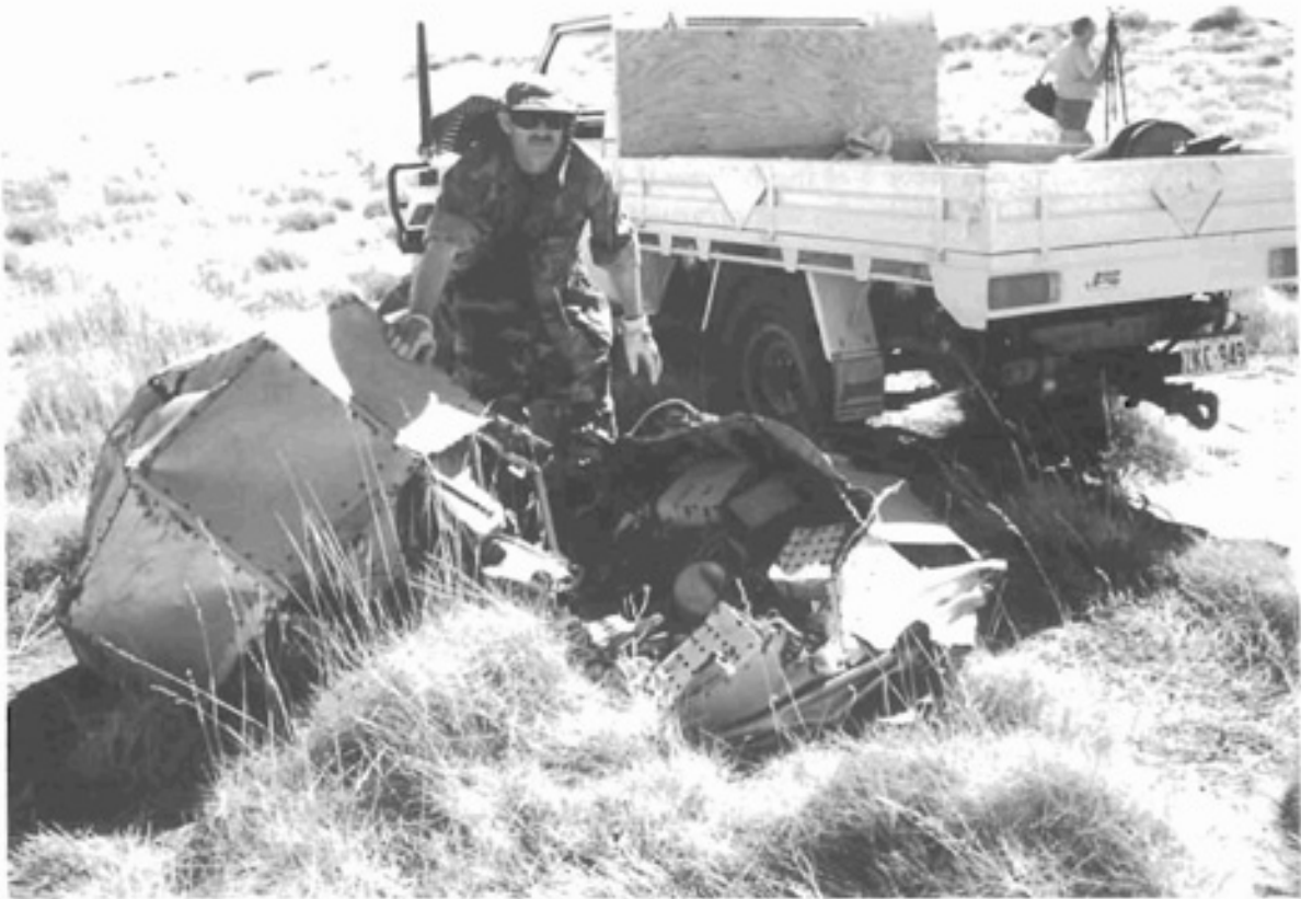
Figure 8 The Europa F-5 dummy satellite, as found. Although the casing had split open on impact, the contents were intact and in good condition. (Roger Henwood)
