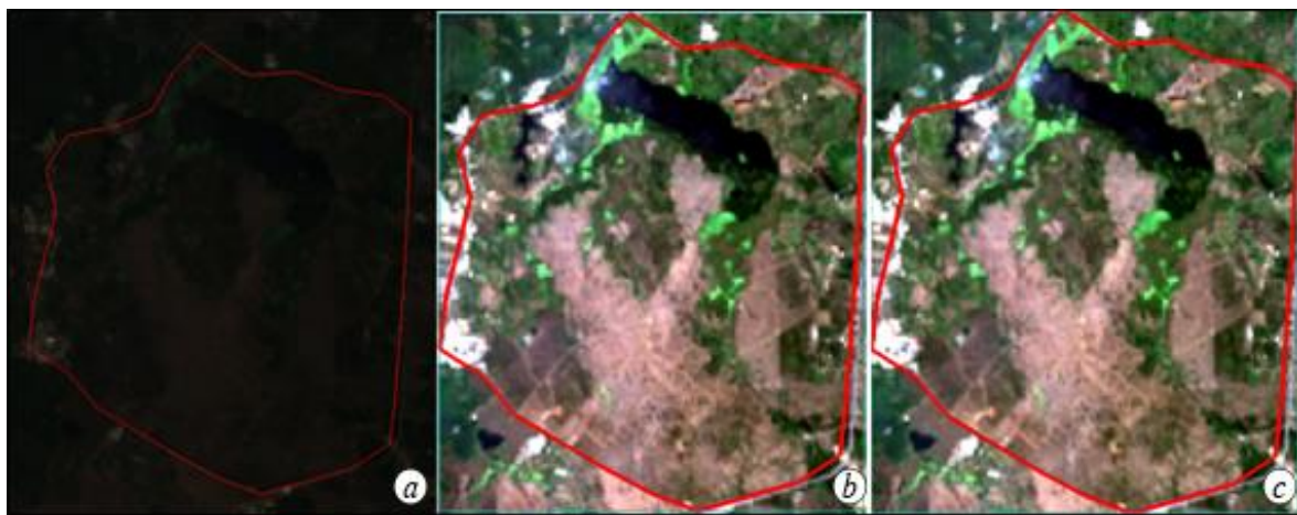
Fig. 2. Processing result of the Landsat image in the ENVI 5.3. Original Landsat image (a). Result image of radiometric calibration (b). Result image of atmospheric correction (c). Differences between (b) and (c) are on pixels level.
