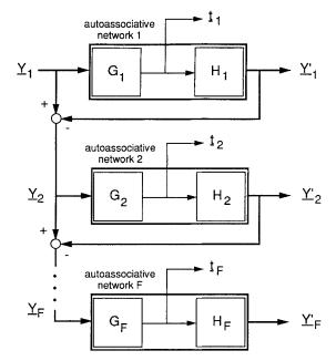
Figure 3. Sequential determination of nonlinear factors by training *F* networks with one bottleneck node each.
