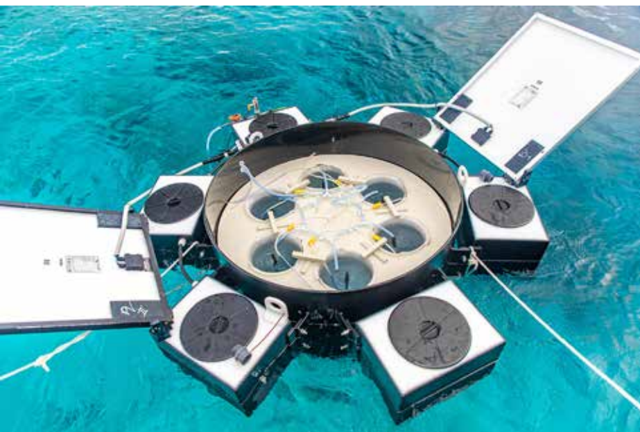
The six incubators are surrounded by the stabilizing boxes in a hexagon shape with the two flaps for the solar panels (not in place). Photo Casper Douma
