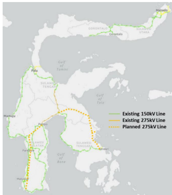
Figure 5.4-3 Outline of the Sulawesi 275kV Green Corridor
