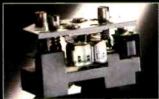
Discrete 3-Head Design Featuring SA Head and Amorphous Head
