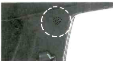
No one looking in can tell there's a Boston 751 system in each of the front doors. Each system includes a 5 1/4" woofer and a flush-mounted 1" Varimount ferrofluid-cooled dome tweeter (installed without the wedge housing). Inset: The 751 two-way component system in front door shown before being covered by the factory panel.
