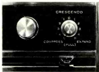
Bogen's novel Crescendo Control is located at the upper right corner of the front panel above the slider volume control.
